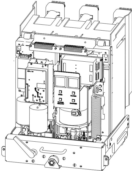
**Figure 4 – Draw Out Circuit Breaker (Front Cover Removed)**
