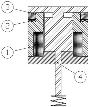
**Figure 2 – Linear (Magnetic) Actuator in Closed Position**
