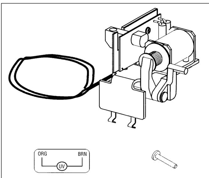
Figure 2-1 Undervoltage Release Mechanism (Handle Reset) and Intermediate Plunger Kit
