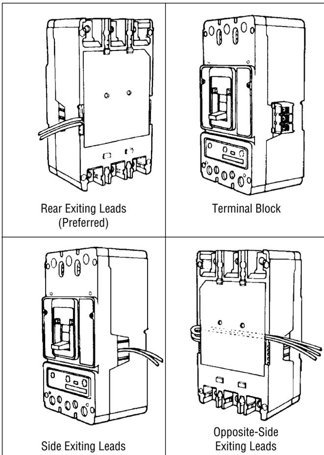
Figure 2-4 Accessory Wiring Options
