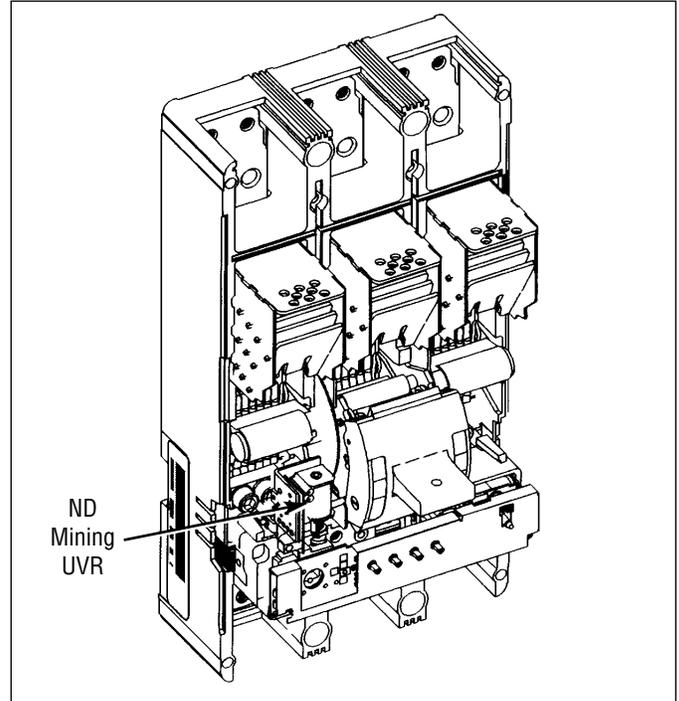
Figure 1-1 Undervoltage Release Mechanism (Handle Reset) Installed in N-Frame Circuit Breakers
