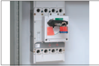
Internal handle can be operated independent of door position and locked-out to meet NFPA 79 and UL 508A disconnect requirements.
