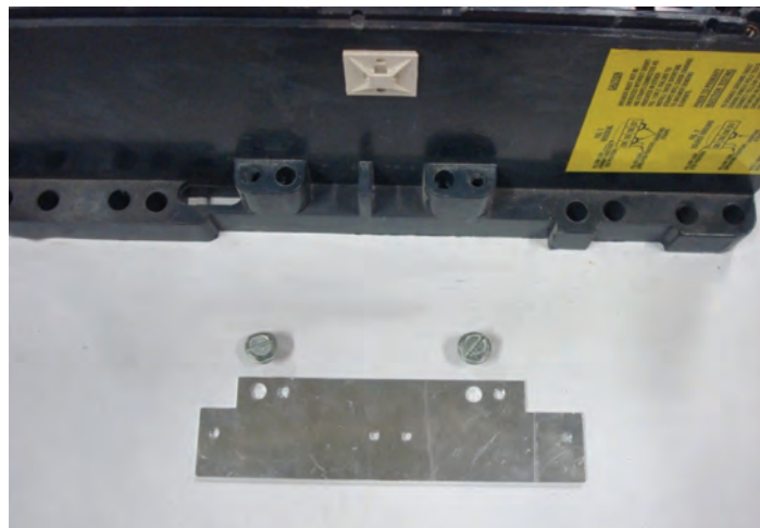
Figure 7. Orientation of the C/D Terminal Block Mounting Plate and Hardware.
