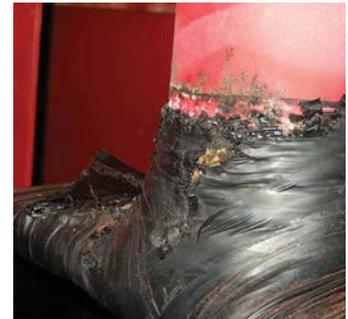
Insulation deterioration within the terminal box motor CP11.
