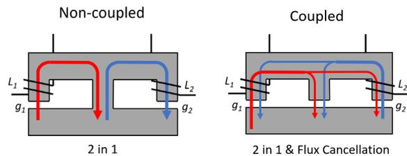
**Figure 2:** Discrete inductors require additional spacing between components compared to integrated inductors which also use common ferrites for greater space savings.
