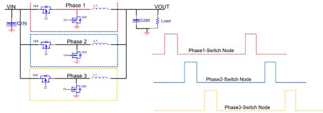
**Figure 1:** A multiphase buck converter can more efficiently handle higher power than a single-phase buck converter of equivalent power output specification.
