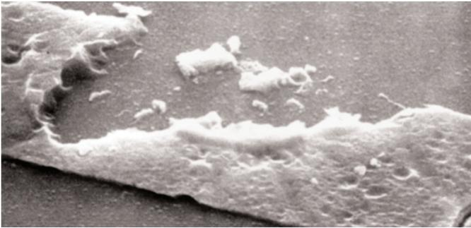
Figure 1. Latent damage due to ESD discharge
