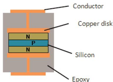
Figure 7. Transient Voltage Suppression construction
