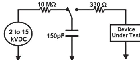
Figure 3. Test setup for Human Body Model
