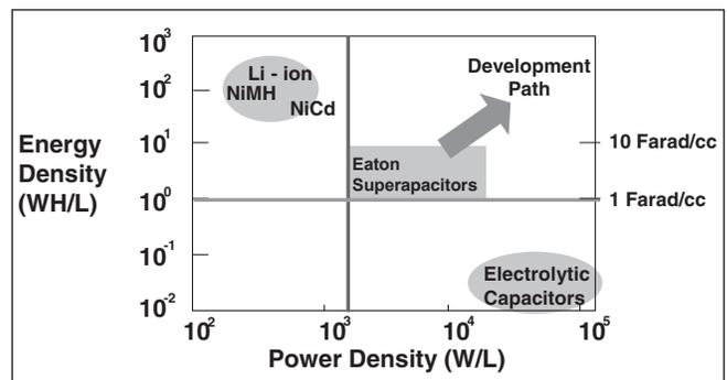
Figure 1. Power density vs. energy density
