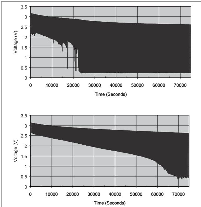
**Figure 2.** 2 AA alkaline batteries (top) to 2 AA alkaline batteries connected in parallel to a single 6F super-capacitor (bottom)
