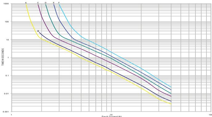
Figure 5. Typical time-to-trip curve
