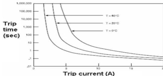
Figure 7. Trip time vs trip current temperature dependency
