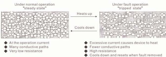
Figure 2. Conductive paths for normal and tripped states
