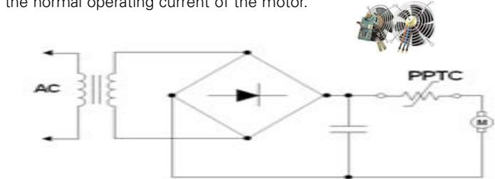
Figure 12. Motor drive protection
