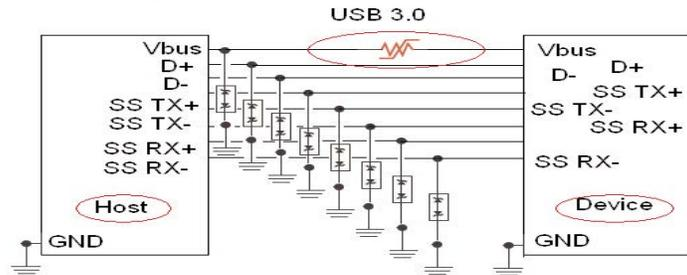
Figure 9. Typical PTC and ESD USB 3.0 application.
