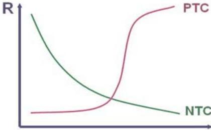
Figure 1. Positive and negative temperature coefficient curves
