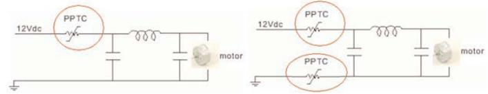
Figure 3. Typical PTC application: Single/multiple supply line protection
