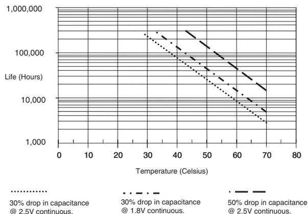
Figure 1. Operating life vs. temperature and charge voltage
