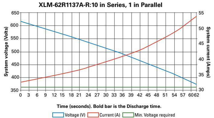
Figure 4. XLM-62R1137A-R calculator output using Figure 5 inputs.
