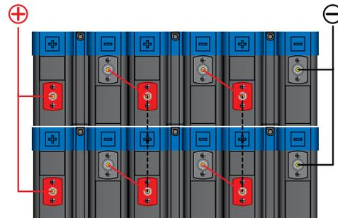
**Figure 8.** 3 Series x 2 Parallel connect modules. In this example, the system would provide 60 kW for 15 seconds at 168 V. Parallel cables (dashed lines) connecting modules in the middle are optional.
