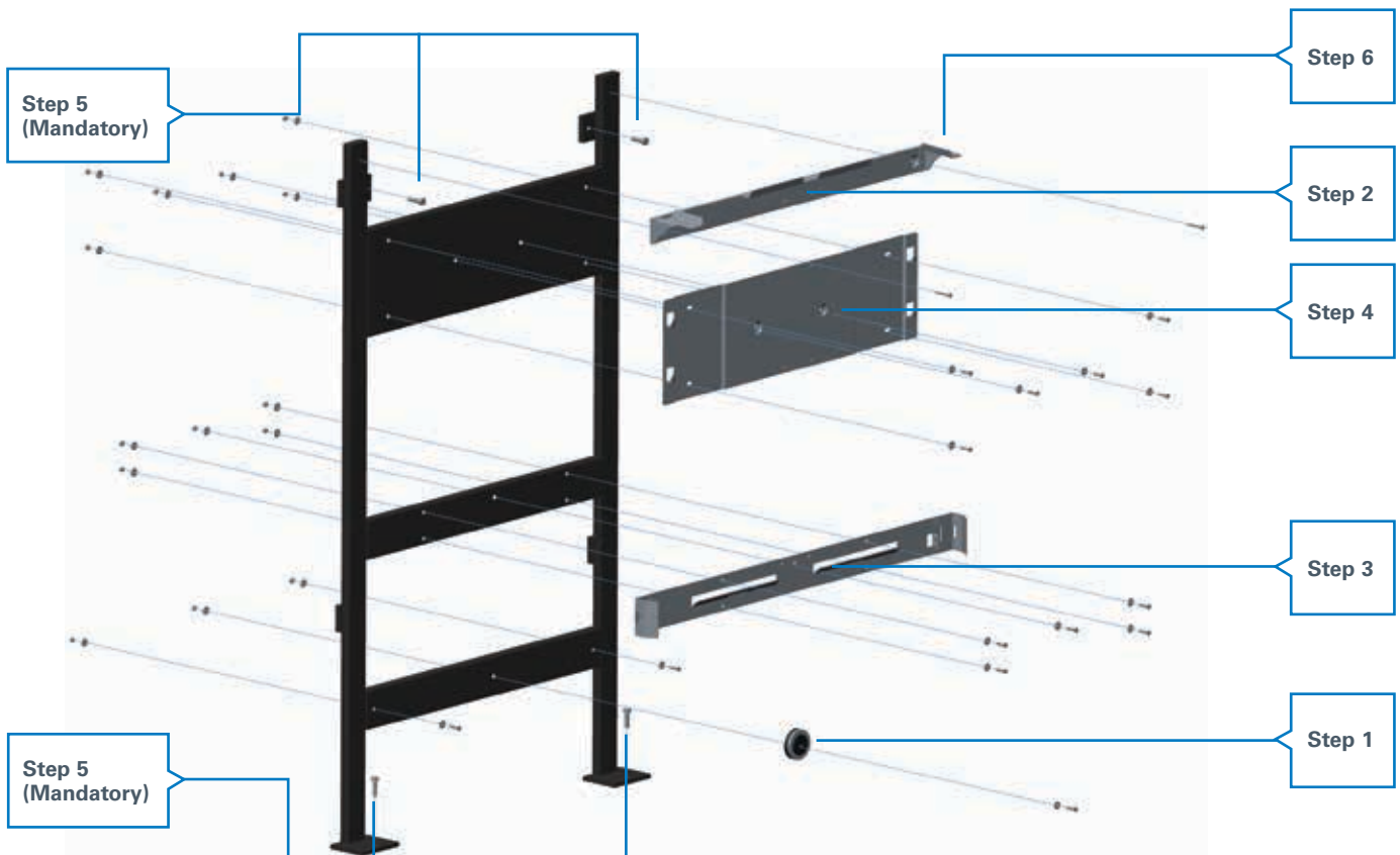
Figure 1: How to fix the floor mounting frame
