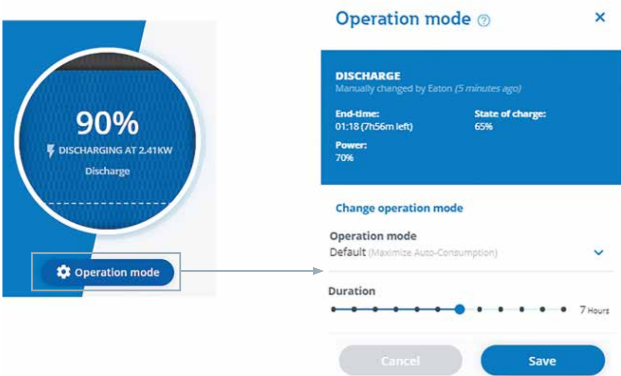
Figure 1: The setup of the operation mode from the "Dashboard"
