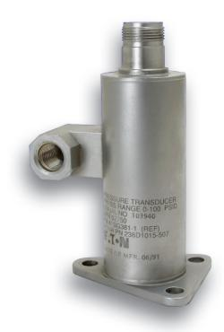
The transducer provides a large low-level output signal proportional to input pressure and voltage. The standard output signal of 0-100 mVDC (with 10 VDC excitation). Alternative outputs for special customer requirements for end point offsets are available. Operating pressure range from 50 to 10,000 psi. Virtually any electrical receptacle and pressure fitting is adaptable to this design.
