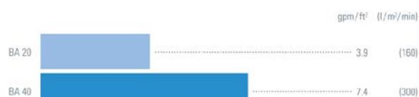
Conditions:  $\Delta p = 14.5$  psi (100 kPa, 1 bar), Medium: Water at 88 °F (20 °C)
