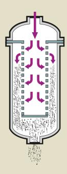
During backwash, triggered by time or pressure differential, a valve switches one station's flow from the inlet header to the drain header and the direction of the flow is reversed in the filter tube, dislodging contaminants from the media surface. The source of the cleaning fluid may be a diversion of process fluids (internal backwashing) or an external source (external backwashing).
