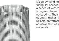
Made by winding a continuous triangular-shaped wire around a series of vertical support stringers, these media require no backing. Their inherent strength makes them ideal for reliable performance with abrasive slurries or fibrous
