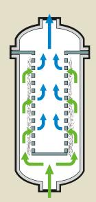
Process liquid flows into the housing inlet at its base and passes across the filter media from the outside inward. Because of this flow path, contaminants collect on the outside of the filter element slowly forming a cake, removing smaller particles.
