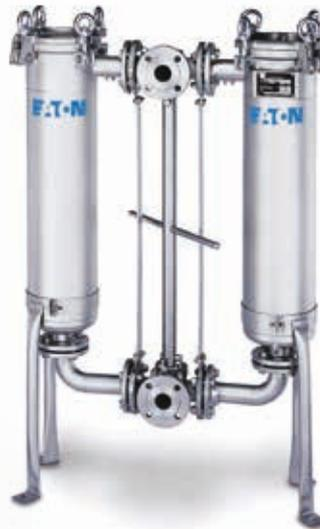
**DUOLINE** multi-bag filter housing system is designed with two single bag filter housings fitted together at the inlet and outlet by a butterfly valve or ball valve. This increases flow capacity and allows the filtration process to run continuously even during filter bag change-outs.
