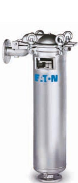
**TOPLINE** single bag filter stainless steel housing is at the top of its class – from its high-performance design to its investment-cast components. The top inlet design requires less headroom and directs liquid flow through the cover which improves sealing, reduces product loss and makes filter bag change-outs cleaner.
