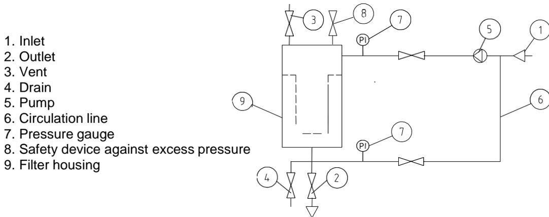
The filter housing shown above is equipped with shut-off devices for discharge and venting. Pressure gauges for measuring the differential pressure are installed in the inlet and outlet connections.
