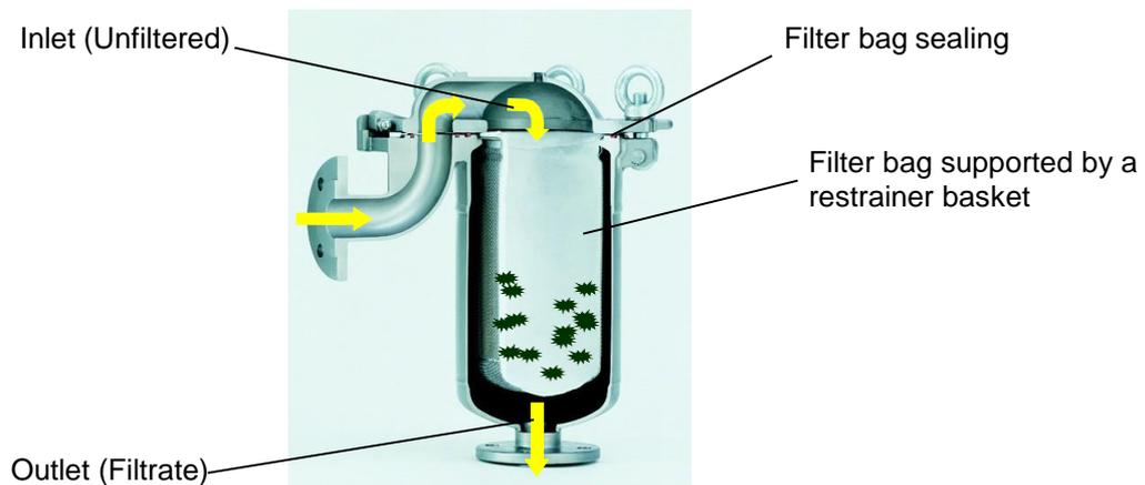
Bag filter housings may contain between 1 and 24 filter bags, depending on type and design. The different designs are adapted to individual applications and may vary greatly. The designs take into consideration operating conditions, materials of construction, connection types and positions, as well as surface finish and operating parameters.
