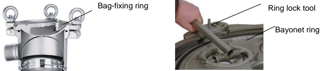
Bag-fixing rings for FLOWLINE and SIDELINE housings have a spring steel band for hold down. The pressure is provided by the cover of the filter housing. It is important that the pressure is applied onto the sealing ring of the filter bag; if it does not the bag-fixing ring may need to be adjusted.
