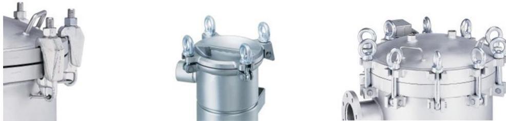
To open the housing: first loosen the eye nuts on the top. The eye nuts can be loosened using a small bar. Where hexagon nuts are used the appropriate wrench should be used. If swing bolts are used the nuts should be loosened enough to allow for them to be swung clear of the cover.
