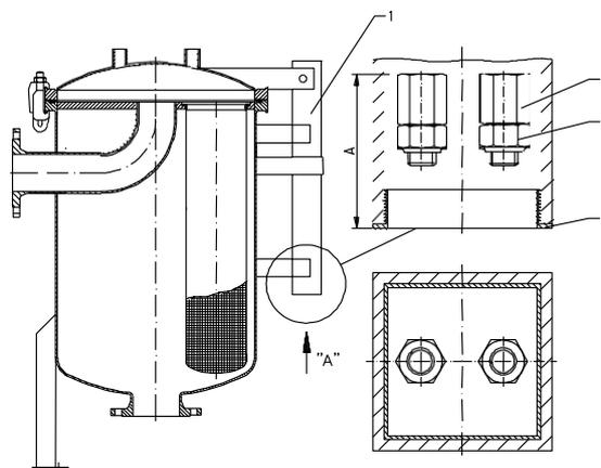
For re-adjustment the dust cap below the spring lift device is to be removed. When viewed from below two threaded bars with hexagon nuts can be seen. Two hexagon nuts are secured with additional self-securing hexagon nuts to guard against misalignment and removal through counters. The counter hexagon nuts must be loosened.
