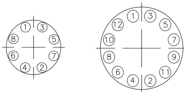
When using maximum allowable torque the bolts are to be tightened in three steps.
