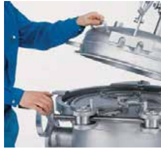
3. Open the cover aided by spring-assisted mechanism.
