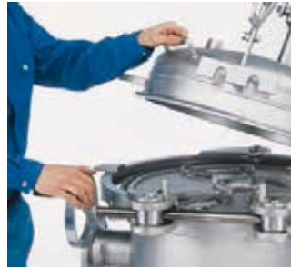
3. Open the cover aided by spring-assisted mechanism.
