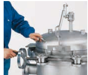
6. Close the V-clamp by rotation of the spindle.
