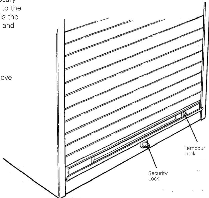
Figure 5. Security lock and tambour lock
