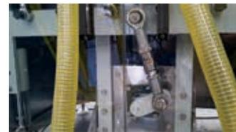
A cam-driven valve system controls the filling volume in IMSB's bottle and pouch filling machines with electronic adjustment.
