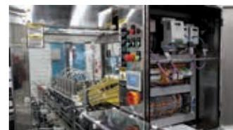
In its new generation of filling machines, PowerXL DA1 frequency inverter control the filling volume and DC1 devices set the optimum speed for the infeed and outfeed conveyors.
