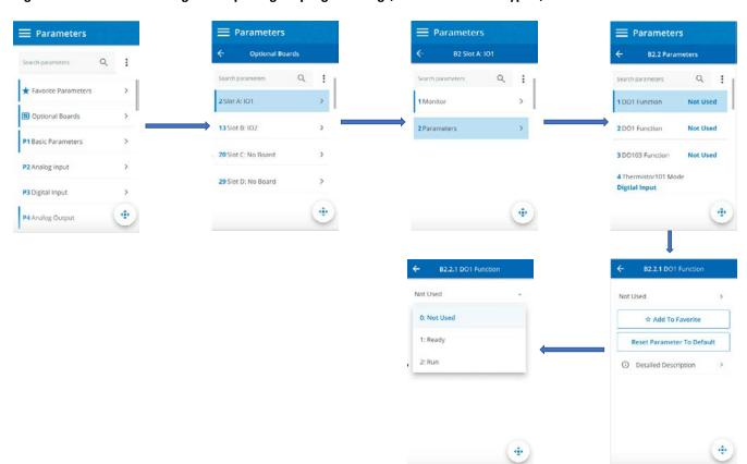
Figure 13. PowerXL DX1 digital output signal programming (via touchscreen keypad)
