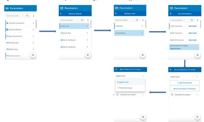
Figure 15. PowerXL DX1 thermistor parameter setting (via touchscreen keypad)
