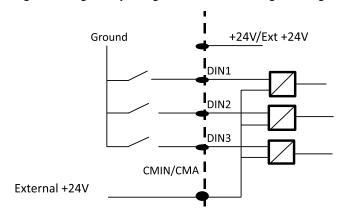
You can also use the positive and negative logic connections with the internal +24 V supply.
