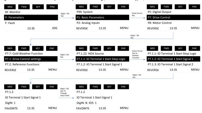
Figure 32. PowerXL DX1 IO5 input board parameter setting (via membrane keypad)
