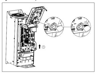
Step 1: Open the control module cover.
