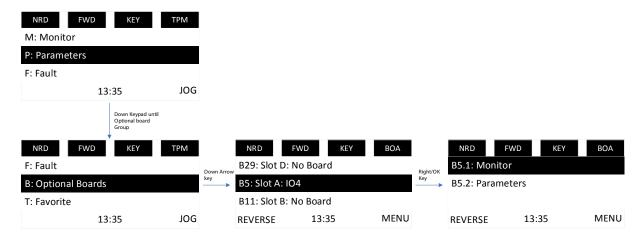
Figure 27. PowerXL DX1 IO4Thermistor board parameter setting (via touchscreen keypad)
