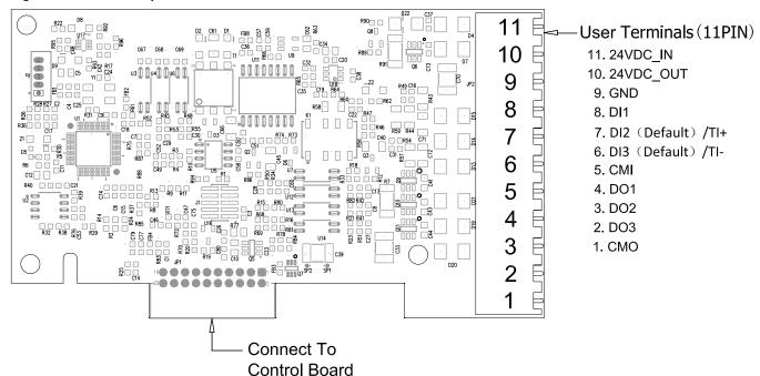
Figure 9. IO1 board wire layout
