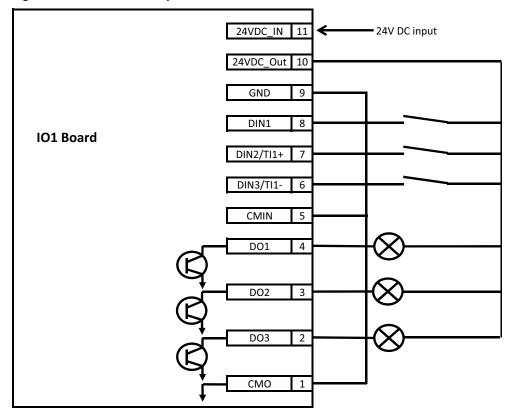
**Note:** If the thermistor inputs are selected, it removes 2 of the digital inputs to be used as the thermistor inputs, inputs DIN2 and DIN3 become thermistor inputs with 4.7K ohm switching point.
