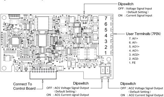
Figure 17. IO2 board wire layout
