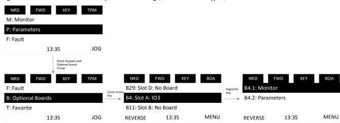
Parameters Parameters Parameters **Optional Boards** B4 Slot A: IO3 Search parameters Search parameters Search parameters Q : ★ Favorite Parameters 4 Slot A: 103 1 Monitor Optional Boards 11 Slot B: No Board 2 Parameters P1 Basic Parameters 20 Slot C: No Board P2 Analog Input 29 Slot D: No Board P3 Digital Input P4 Analog Output
