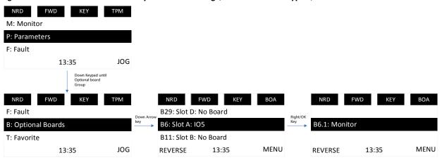
Parameters **Parameters** Parameters **Optional Boards** B6 Slot A: IO5 : \* Favorite Parameters 6 Slot A: 105 1 Monitor Optional Boards 11 Slot B: No Board P1 Basic Parameters 20 Slot C: No Board P2 Analog Input 29 Slot D: No Board P3 Digital Input P4 Analog Output
