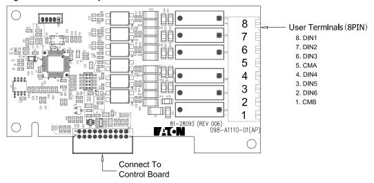
Figure 29. IO5 board wire layout
