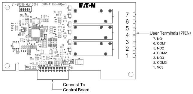
Figure 21. IO3 board wire layout
