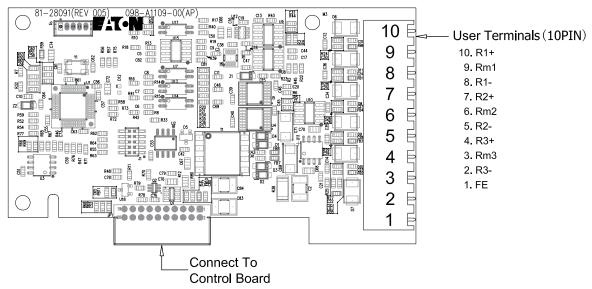
Figure 25. IO4 board wire layout—options for wiring the sensor
