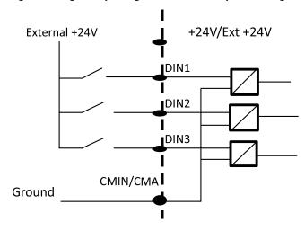
Figure 6. Digital input signal conversion-negative logic
