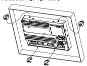
Step 3: Torque all fasteners to 6.17lb-inch (0.7N-M) Over torque may cause damage to the operator interface housing.
