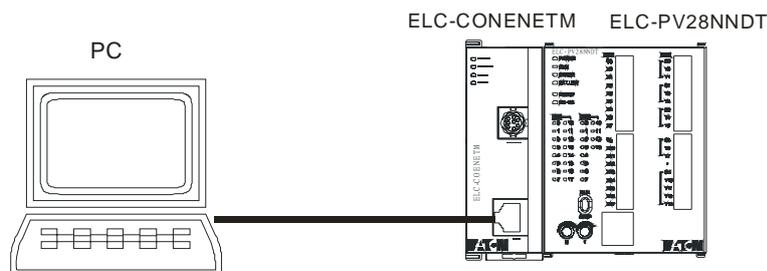
(Note: the default IP address setting for the ELC-COENETM module is IP address = 192.168.1.5. The PC IP address and network mask need to be set up to reside on the same network as the ELC-COENETM)
