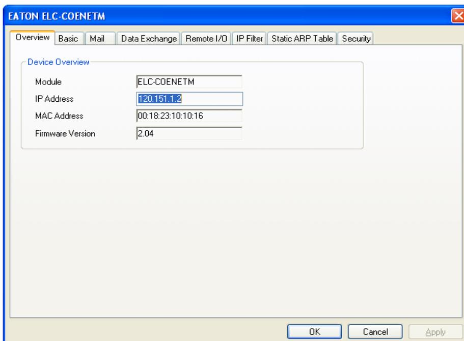
The Overview window displays specifics about each module. The Basic tab allows the IP address to be changed as well as the subnet mask and gateway address. This is also where the IP address can be made Static or DHCP. Be sure Modbus TCP is enabled in the bottom left portion of the screen. When finished, the Basic tab looks like the following for this example:
