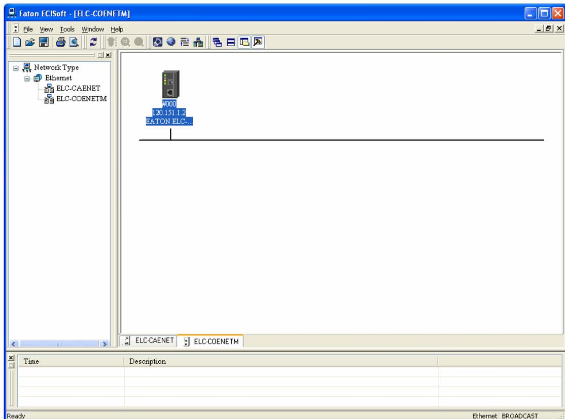
Note the two tabs at the bottom left of the main window. Both modules have been found and each type of module is located in a separate tab. Click the tab for the ELC-CAENET module, then double click its icon to open its configuration pages as follows:
