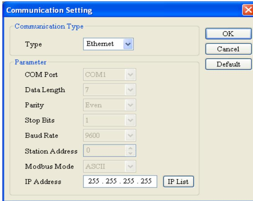
Click OK after selecting Ethernet for the Type. Then in ECISoft, click the IP “magnifying glass” and the software will search for all ELC Ethernet devices connected to the same Ethernet switch. When complete, the following screen will be displayed:
