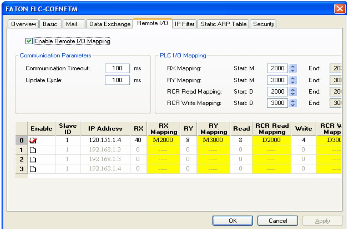
Note that the data is mapped to addresses in the ELC-PV controller connected the ELC-COENETM module. These addresses may be changed under PLC I/O Mapping in the upper right portion of this page. Enter different starting addresses and the end address will change based on the amount of data for each. The valid ranges for the M bits and D registers are as follows:
