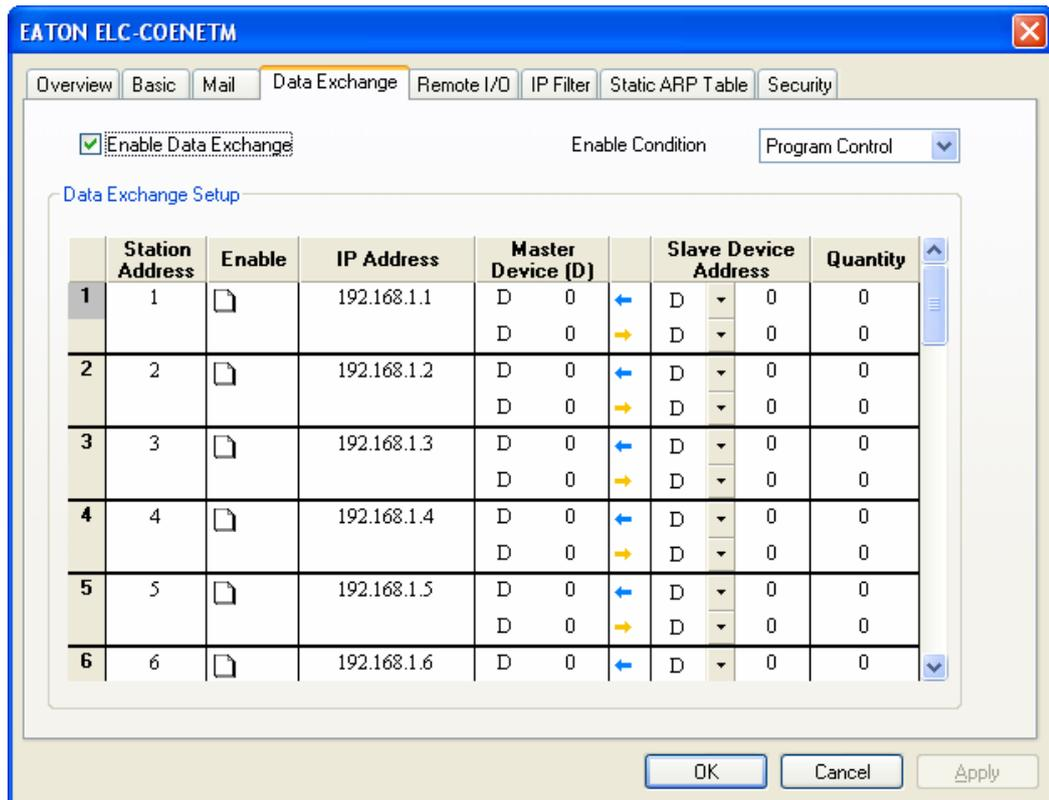
In the top right portion of the screen, select “Always Enable” or “Program Control” to determine how the messages will be triggered. Always Enable means the Ethernet module will continuously send the messages. It will get the data for write messages from the attached ELC-PV controller and send it to the D-registers selected for the Slave controller. For read messages it will read the data from the Slave controller and store the data in the selected D-registers in the local, attached controller.
