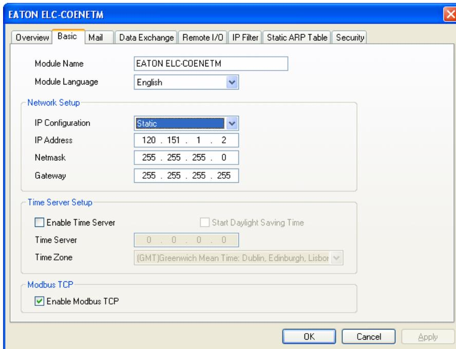
Configure the other Ethernet module in the same manner. The Ethernet module at IP address 120.151.1.4 will only require setting up the IP address, subnet mask and optional gateway address. It will only be receiving messages from the other Ethernet module.
