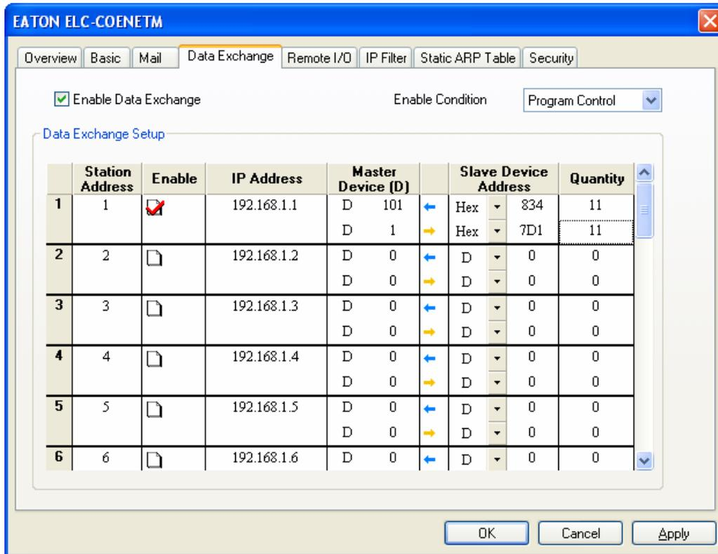
After the ELC enters run mode, it will begin exchanging data from its D registers with the modbus registers in the Drive.
