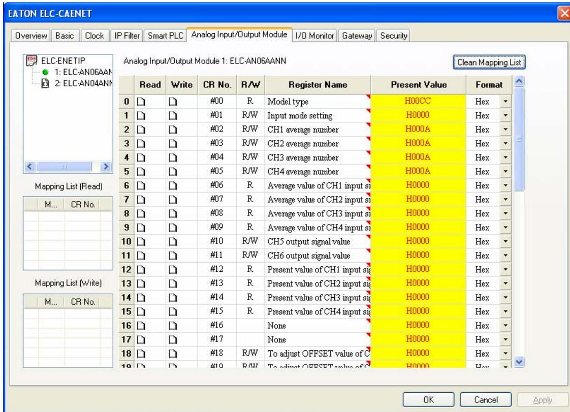
The upper box on the left displays the two analog modules. Click the module to be mapped so the green dot appears to its left. The AN06AANN is selected, so we can begin mapping its data. For this example, the following data will be mapped for this module:
