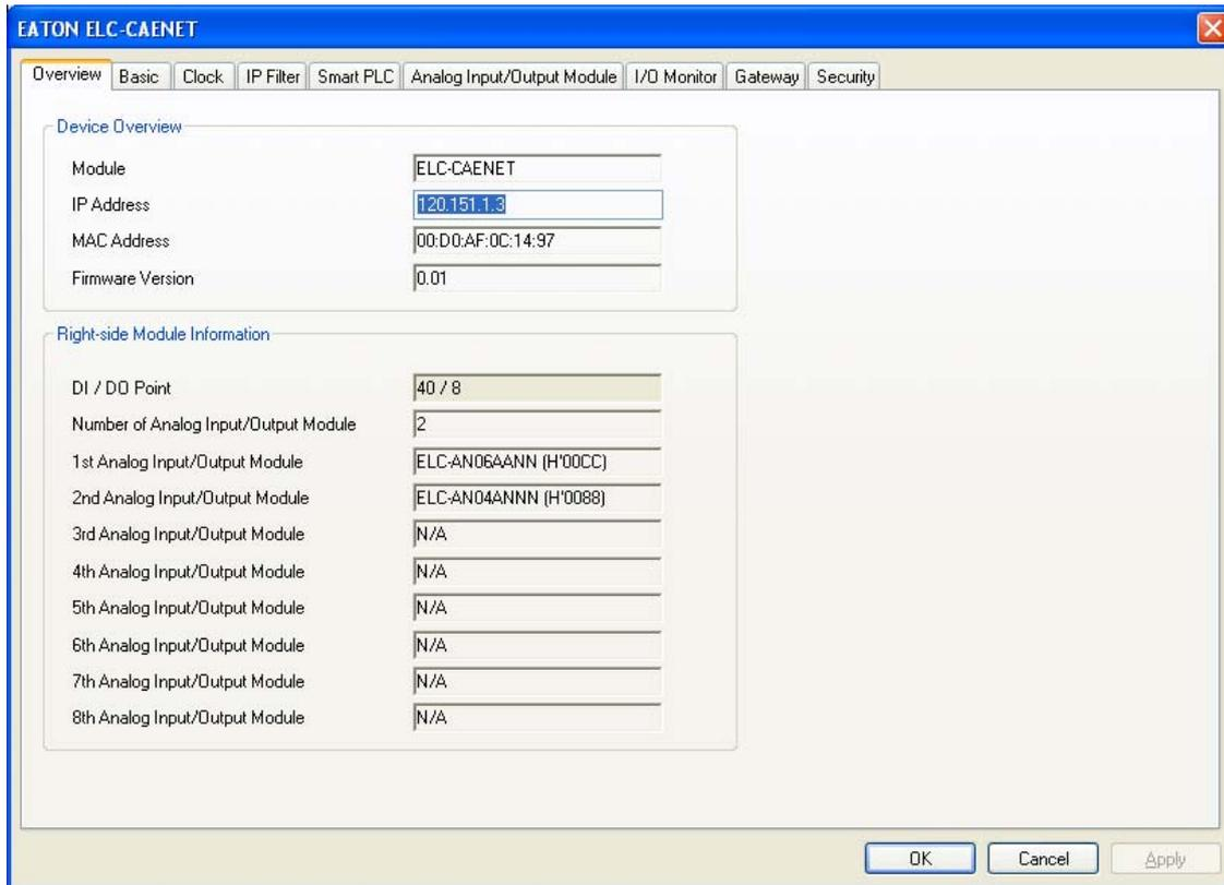
The Overview window displays specifics about each module. The Basic tab allows the IP address to be changed as well as the subnet mask and gateway address. This is also where the IP address can be made static or DHCP. When finished, the Basic tab looks like the following for this example:
