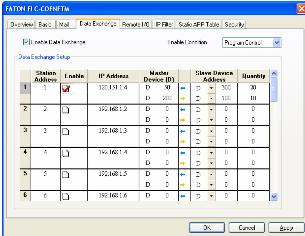
Enable Data Exchange must be selected before any messages can be configured.
