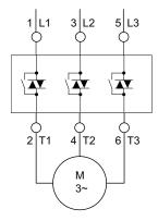
For each start, the length of time the SCRs are conducting current as well as the magnitude of that current determine how hot the SCRs will get. Between successive starts the SCRs must cool down to avoid exceeding their thermal limits. **Appendix C** gives the S801+'s application ratings for various starting conditions. Staying within these specified limits will aid in avoiding over temperature trips.
