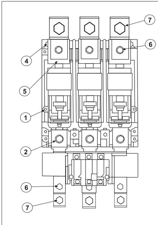
Fig. 8 Torquing Locations
