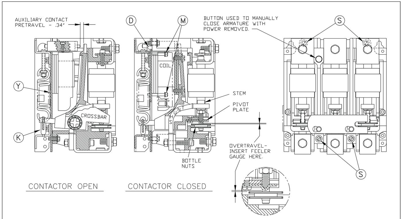
Fig. 9 Contactor Portion of a V200 Motor Controller
