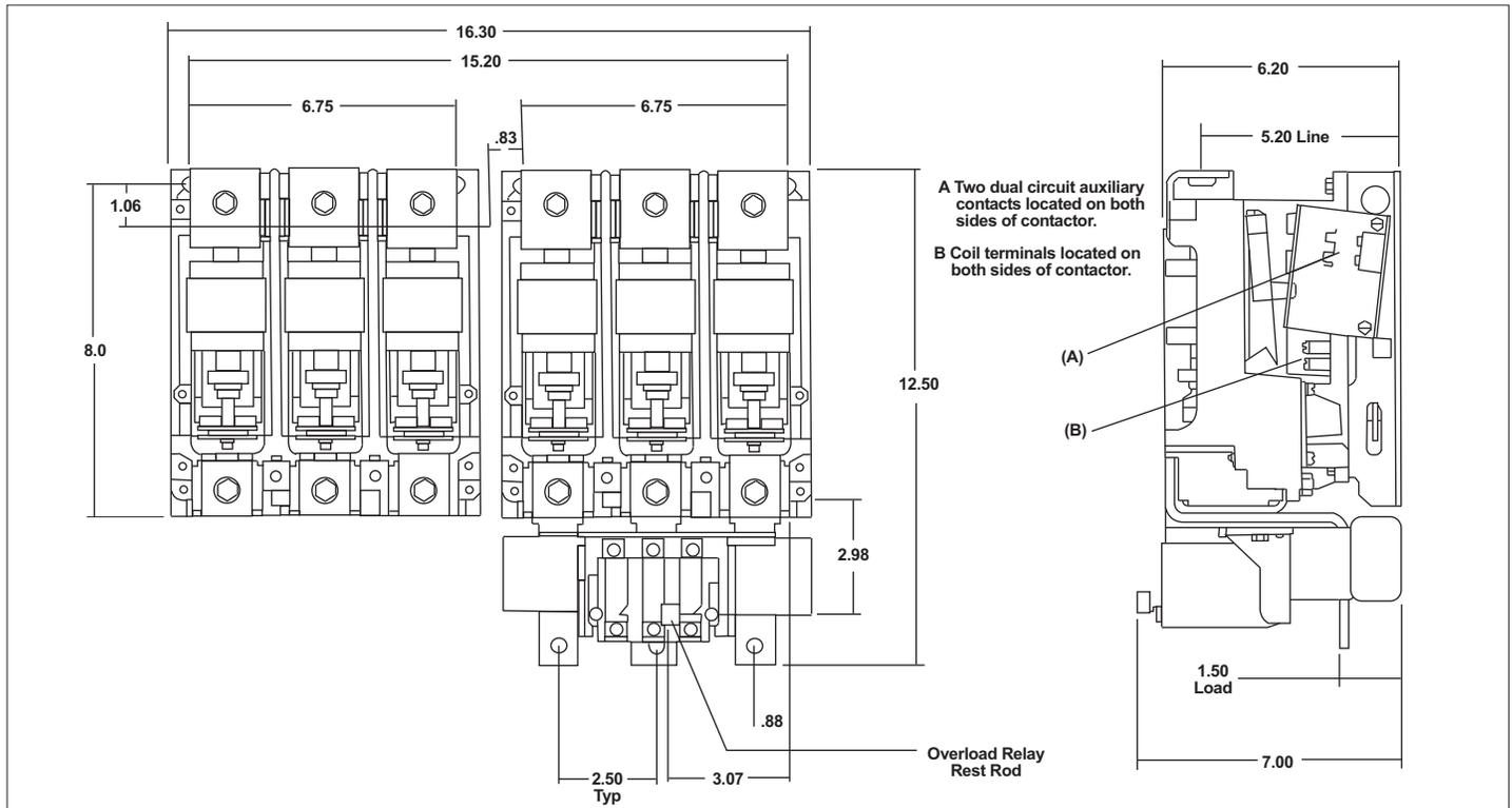
Fig. 3 Reversing Controller (V210) Dimension Drawing (Dimensions in inches)
