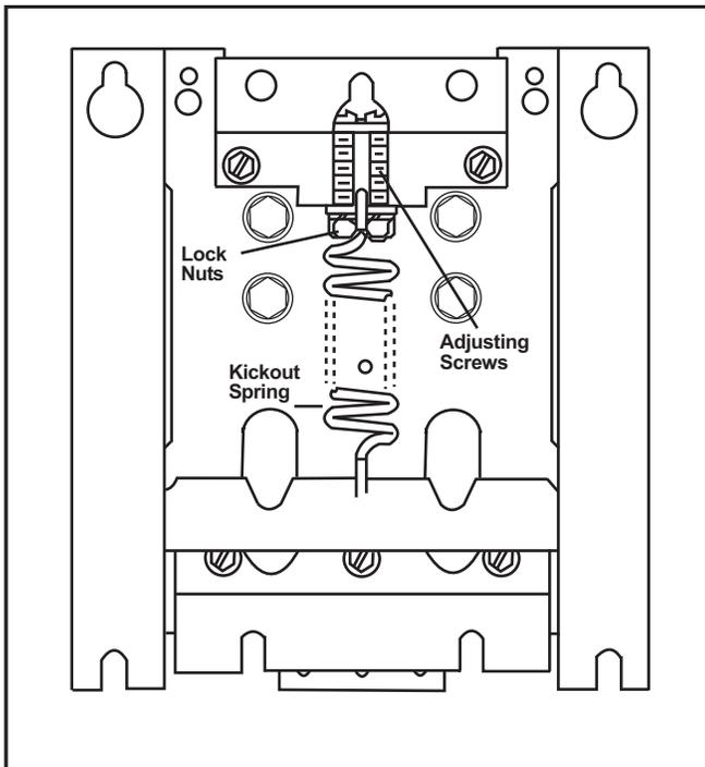
Fig. 10 Kickout Spring
