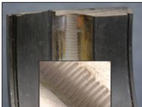
Figure 2. Fluting in Bearing Race Caused by Bearing Currents [2]
