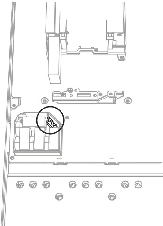
**FS7 only:** Locate the DC grounding busbar between connectors R- and U and detach the busbar from the frame by undoing the M4 screw. See figure below.
