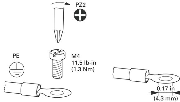
The ground connection is connected directly with the cable clamp plates.
