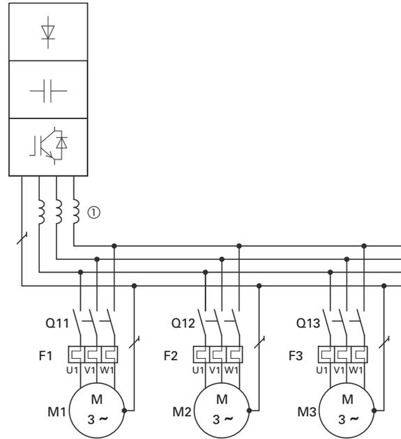
Connecting motors in parallel reduces the load resistance at the frequency inverter output. The total stator inductance is lower and the leakage capacity of the lines greater. As a result, the current distortion is greater than in a single-motor circuit. To reduce the current distortion, you should use motor reactors (see **1** in figure above) in the output of the frequency inverter.
