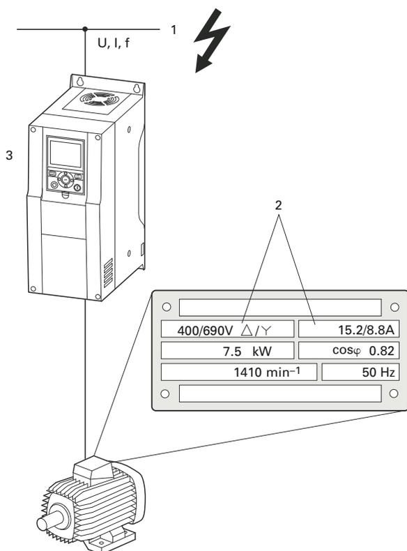
When connecting multiple motors in parallel to the output of a frequency inverter, the motor currents are added geometrically—separated by effective and idle current components. When you select a frequency inverter, make sure that it can supply the total resulting current. If necessary, for dampening and compensating the deviating current values, motor reactors or sinusoidal filters must be connected between the frequency inverter and the motor.
