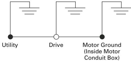
**IMPORTANT:** Improper grounding could result in damage to the motor and/or drive and could void warranty.
