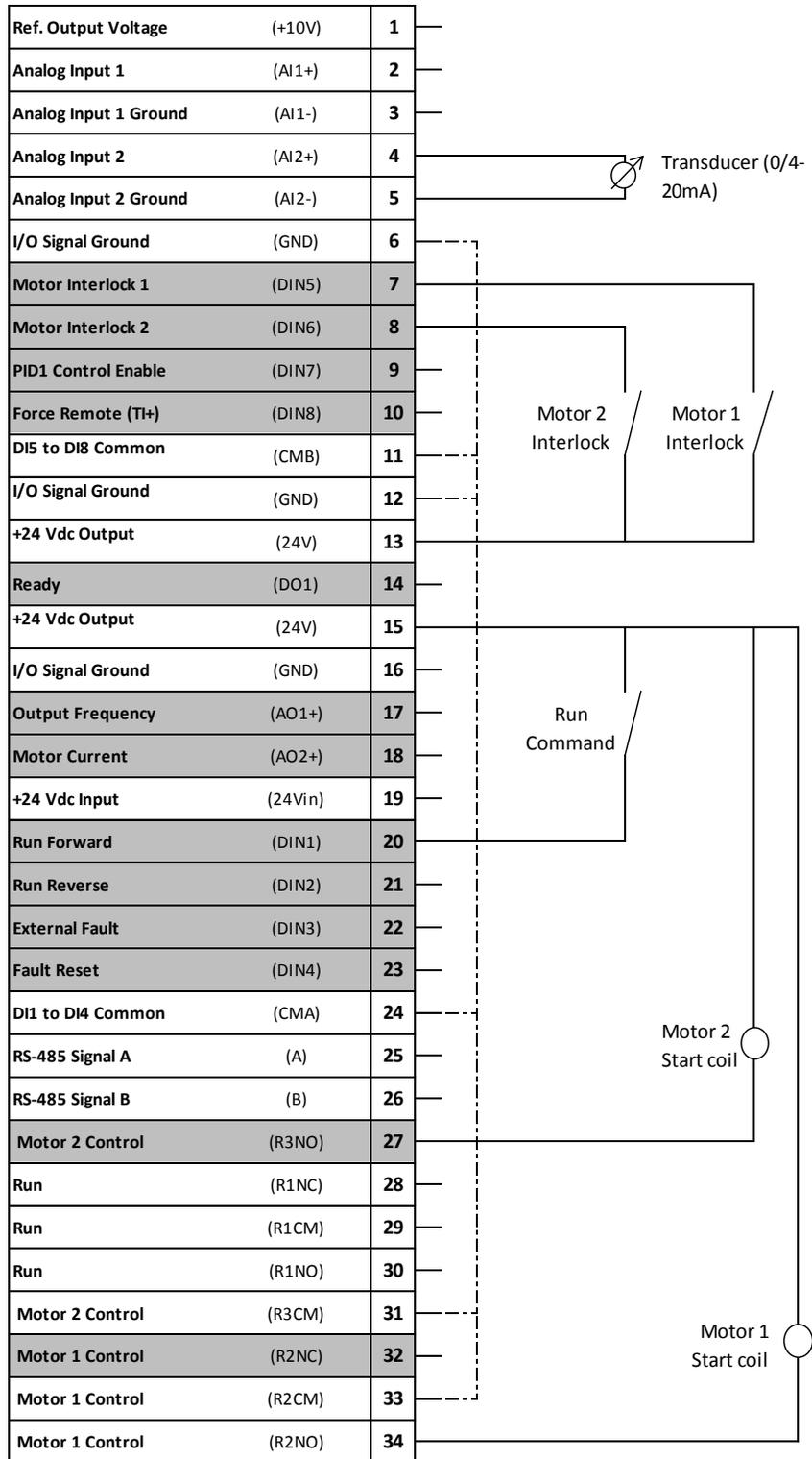
Figure 1: Multi-Pump Two Motor Control Scheme
