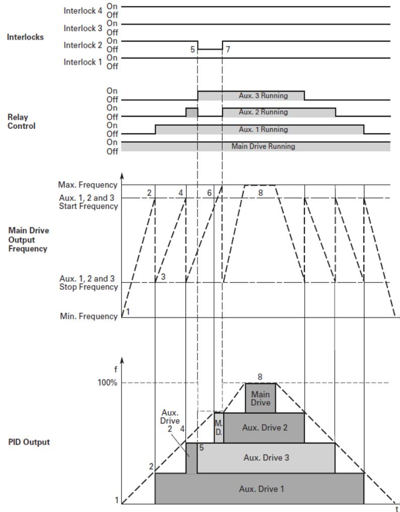
Figure 3: Multi-Pump Interlock Control Scheme
