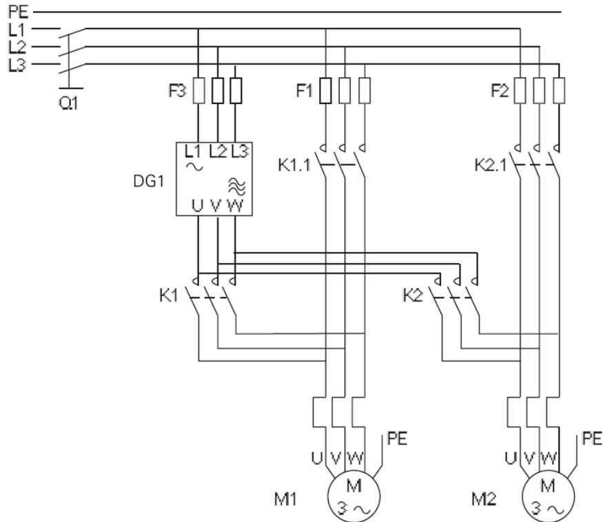
**Figure 2: Multi-Pump Two Motor Power Wiring**
