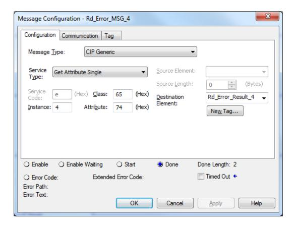
The result of the Message read that is requesting the Motor Current (PNU Index 504) or any other parameter (PNU Index number) is shown in the RD\_Data\_Result in the attached program. This tag includes the command header information as well as the raw data for the requested PNU Index number.
