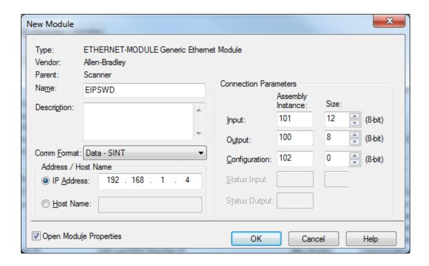
Click OK, then enter an RPI time on the Connection Tab and click OK again. Generic I/O tags will be created with the name "EIPSWD" in the Controller tag area.
