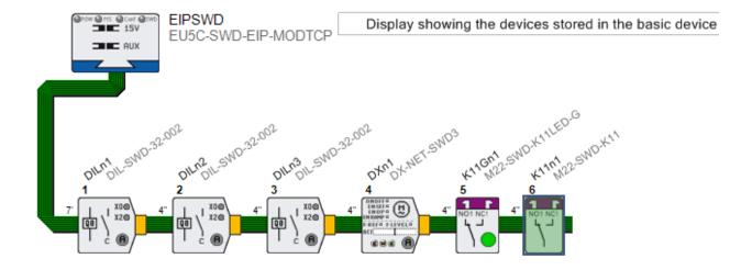
Note that the DC1 Drive (DX-NET-SWD3) is node 4 on the Smartwire network. This information will be needed when using Message instructions in RSLogix5000 to read the motor current via Acyclic/Explicit messages.
