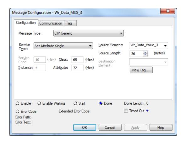
Command written to the DC1 drive for this example, to set it up to read the motor current in a subsequent message read. Refer to page 77 in publication MN04012009Z for a complete description of each value.
