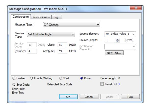
2. Another Set Attribute Single message, sending 1 byte of data containing the length of the subsequent Smartwire command. The length is 10 bytes.
