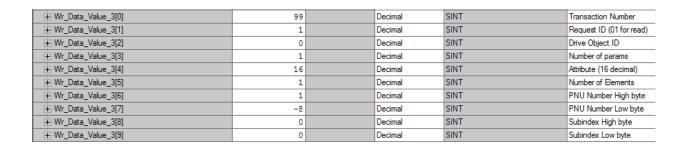
The PNU Index number is from the DE1/DC1 Smartwire manual. Note which is the high byte and which is the low byte. The program provided with this application
