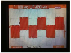
Figure 2 - PWM waveform taken at a motor with dV/dT filter
