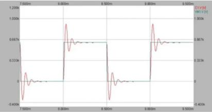
Figure 1 - voltage pulse to the motor and voltage ringing due to impedance mismatch.
