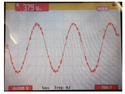
Figure 6: With Sine Filter
