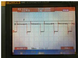
Figure 4: With dV/dT filter
