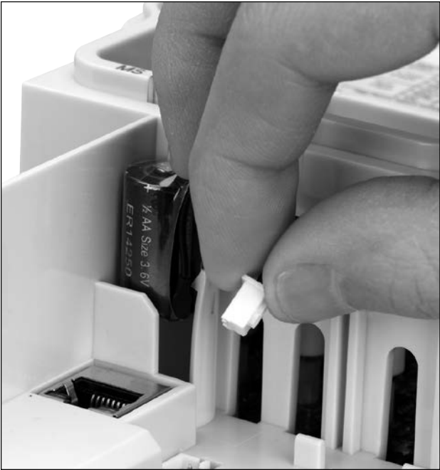
Figure 1. RTC battery connection
