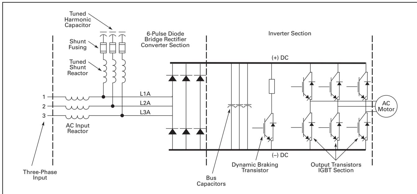
Figure 31.0-12. Enclosed Drive with Integrated Passive Filter
