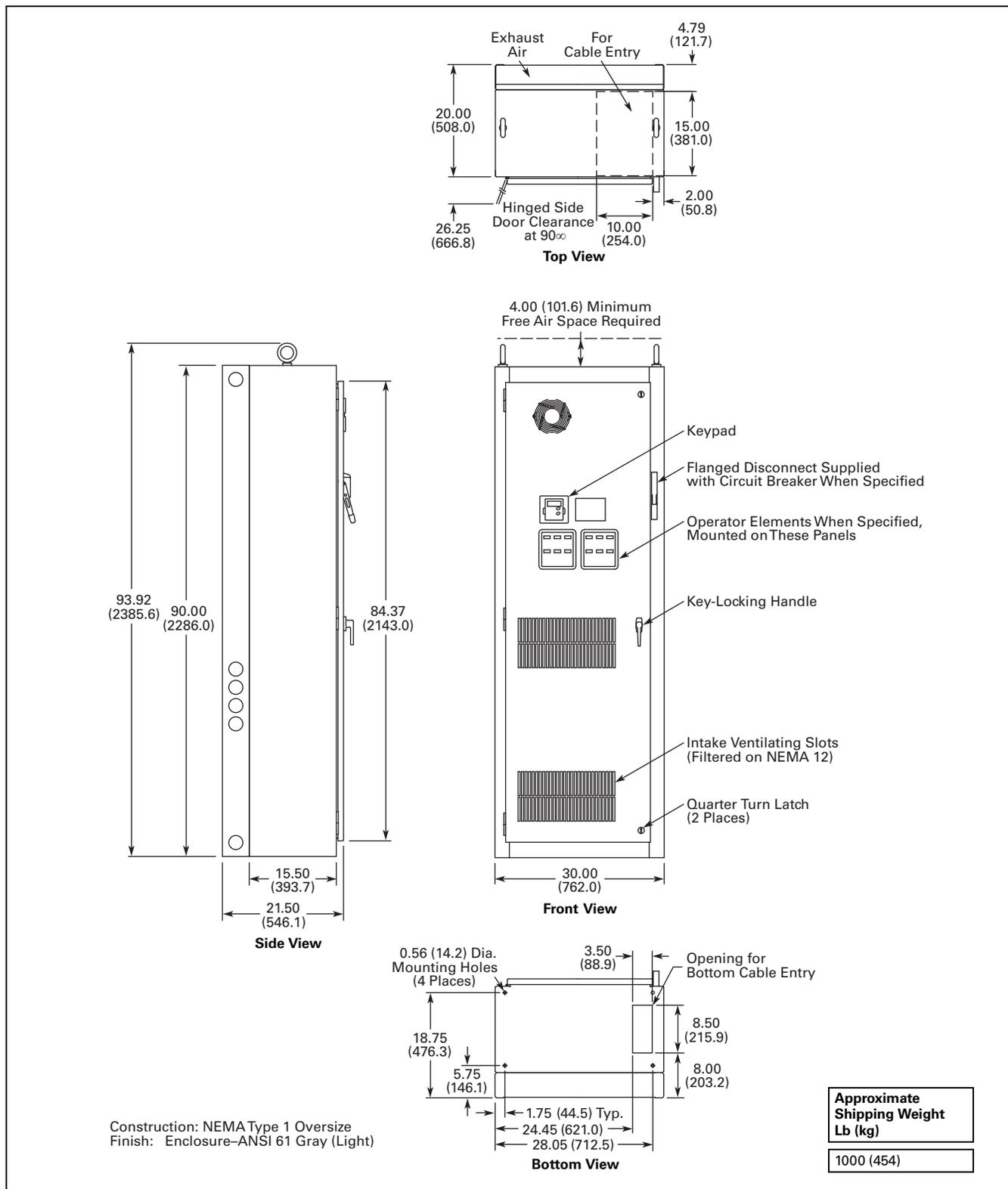
Figure 31.2-40. Enclosure Size 7—Approximate Dimensions in Inches (mm)
