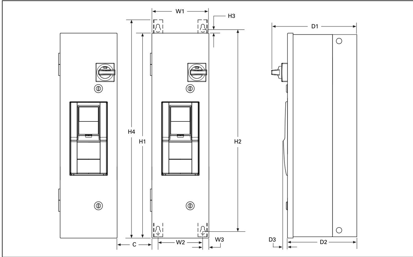
Figure 31.3-6. H-Max Series IntelliPass and IntelliDisconnect Drives
