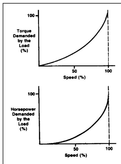
Figure 31.0-3. Variable Torque Load
