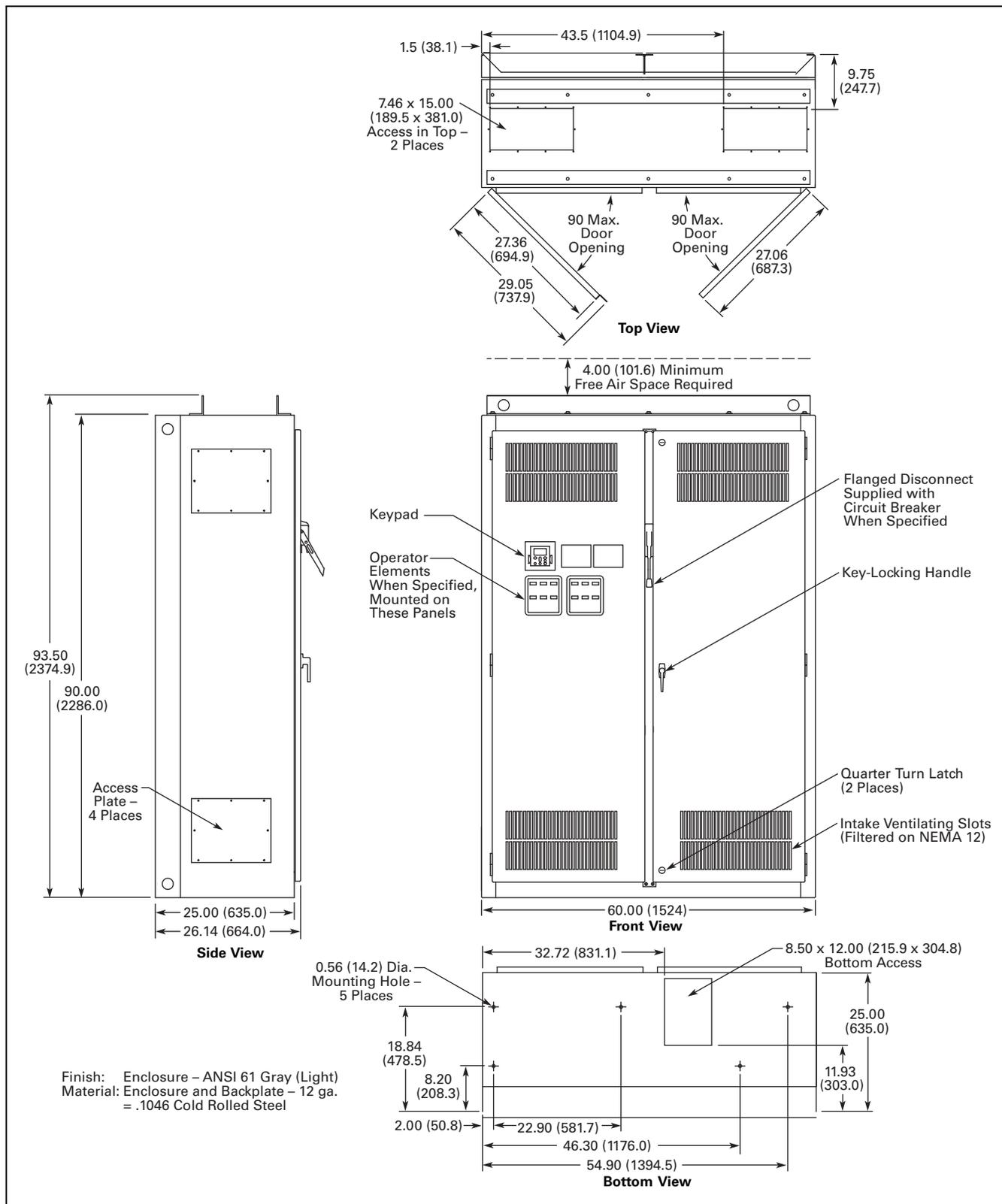
Figure 31.2-45. 300–400 hp I<sub>L</sub> and 250–350 hp I<sub>H</sub>—Approximate Dimensions in Inches (mm)
