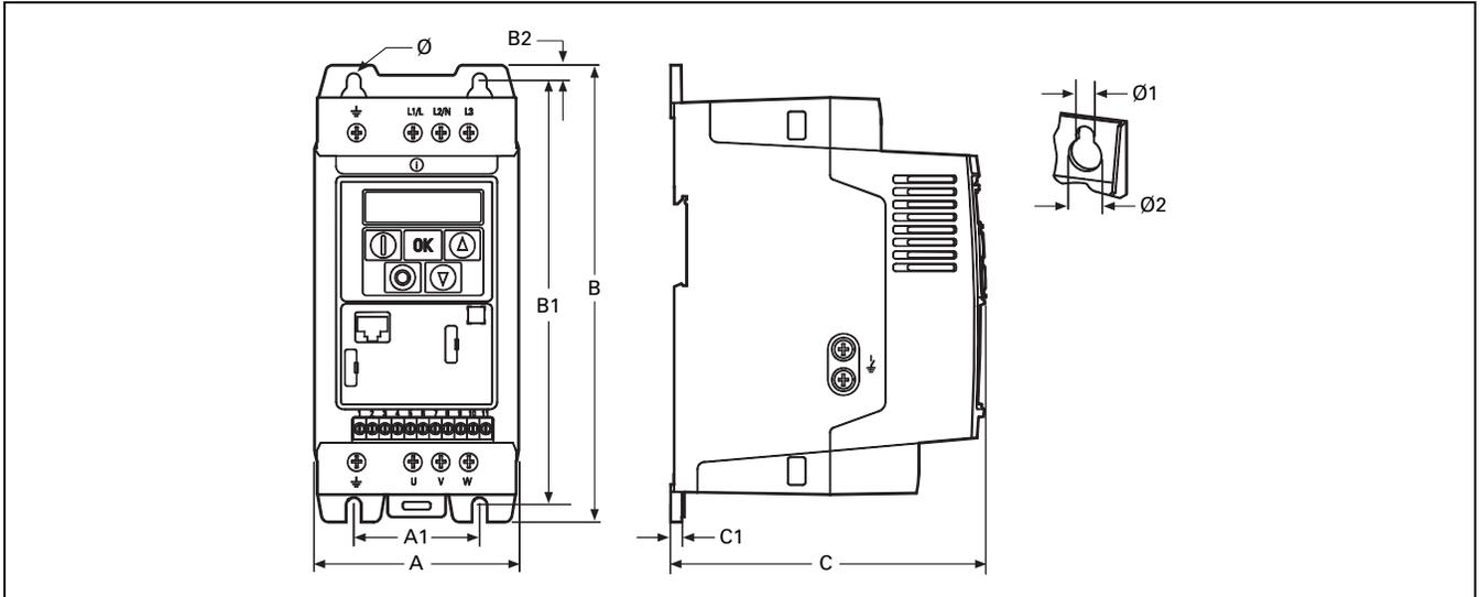
**Figure 31.1-2. DC1, Sizes FS1–FS4, Degree of Protection IP20/NEMA 0**
