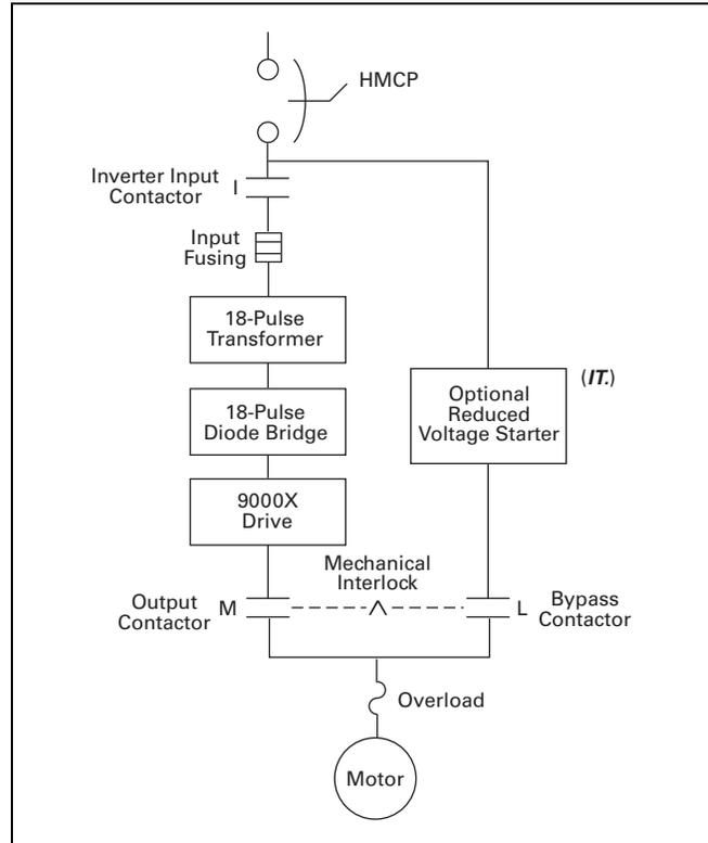
Figure 31.2-49. Power Diagram 25–250 hp  $I_L$  and 25–200 hp  $I_H$  with Bypass
