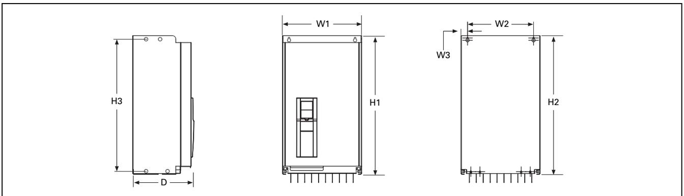
**Figure 31.3-3. H-Max Series Frames FS8 and FS9**
