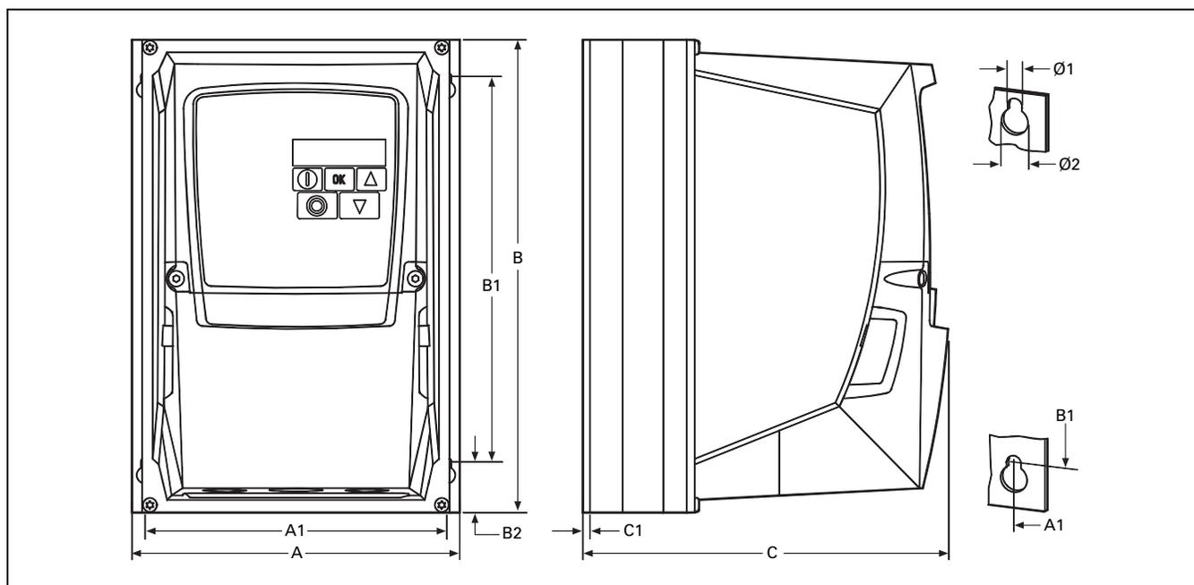
Figure 31.1-3. DC1, Sizes FS1–FS3, Degree of Protection IP66/NEMA 4
