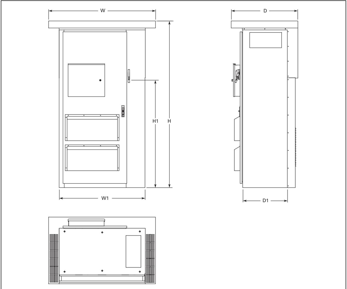
**Figure 31.2-39. Enclosure Size F—Approximate Dimensions in Inches (mm)**
