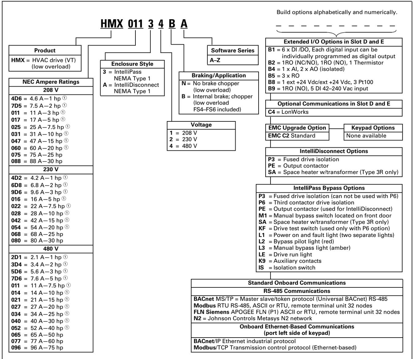
① DB chopper standard frames FS4–FS6 for USA application. 1.5–40 hp, 2.1–52 A, 480 Vac; 1–20 hp, 4.2–54 A, 230 Vac; 1–20 hp, 4.6–60 A, 208 Vac.
