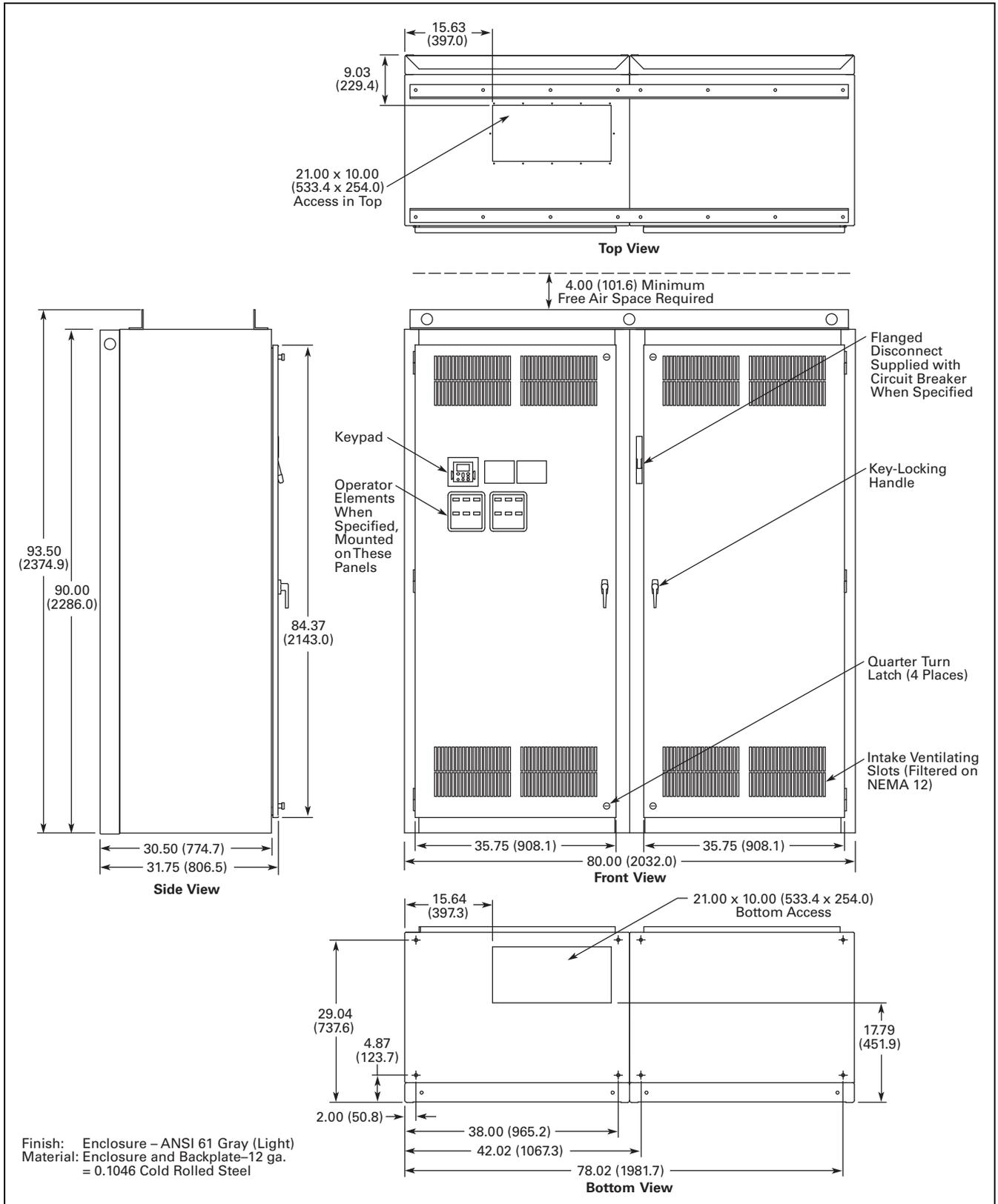
**Figure 31.2-46. 500–600 hp I<sub>L</sub> and 400–500 hp I<sub>H</sub>—Approximate Dimensions in Inches (mm)**
