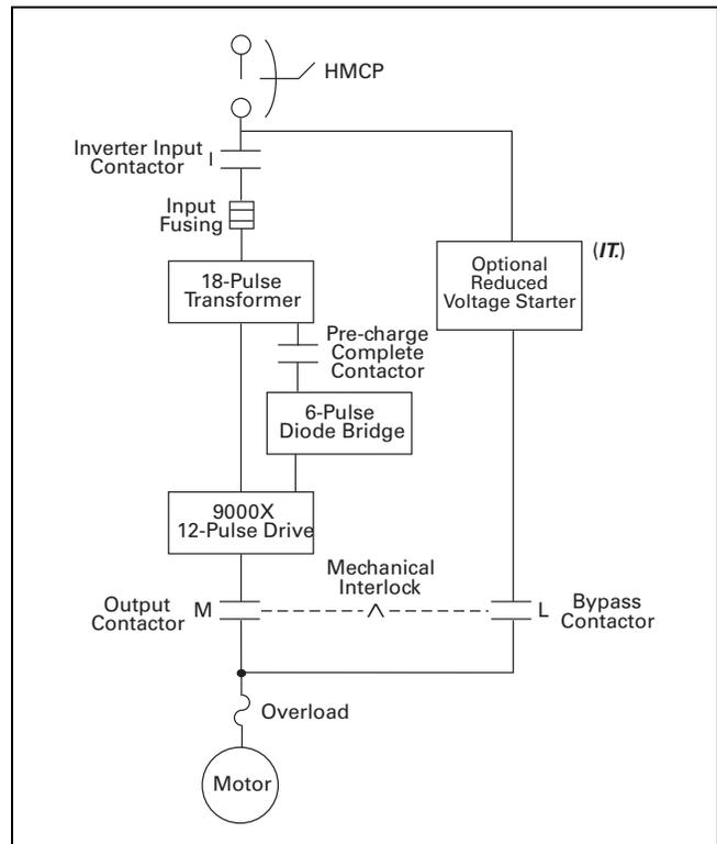
Figure 31.2-50. Power Diagram 300+ hp  $I_L$ /250+ hp  $I_H$  with Bypass
