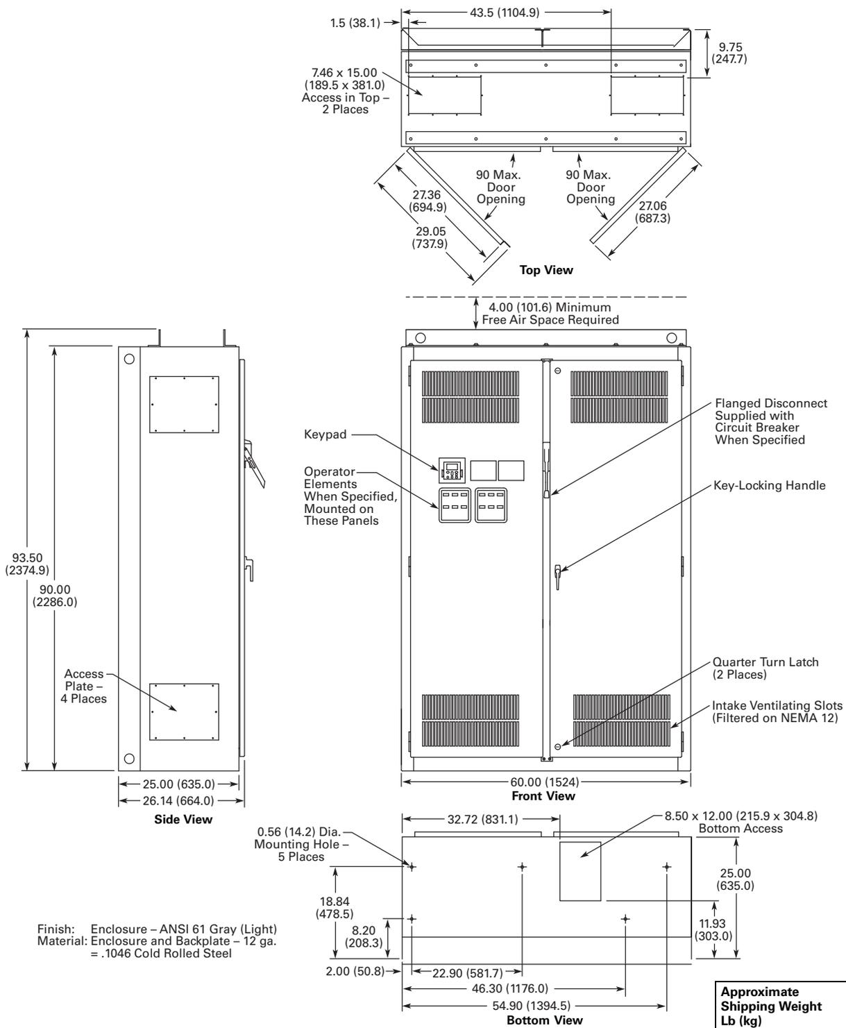
Figure 31.2-42. Enclosure Size 9—Approximate Dimensions in Inches (mm)
