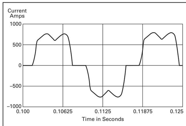
Figure 31.0-8. 100 hp Six-Pulse Nonproductive Harmonic Current
