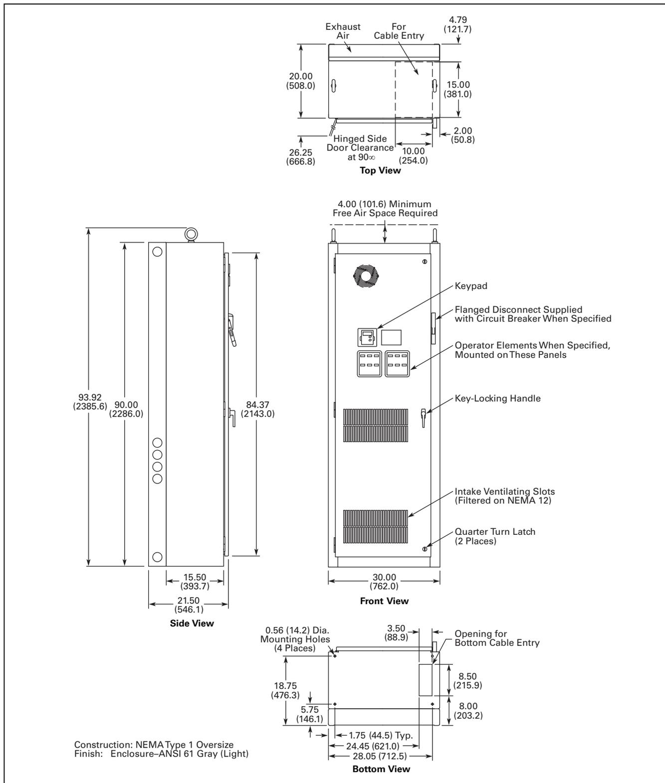
Figure 31.2-43. 25–150 hp I<sub>L</sub> and 25–125 hp I<sub>H</sub>—Approximate Dimensions in Inches (mm)
