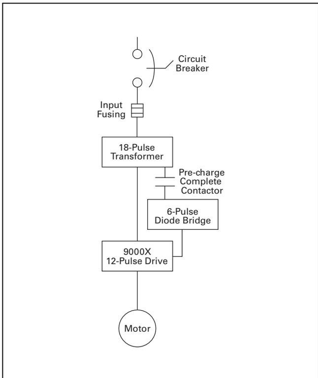
Figure 31.2-48. Power Diagram 300+ hp  $I_L$  and 250+ hp  $I_H$
