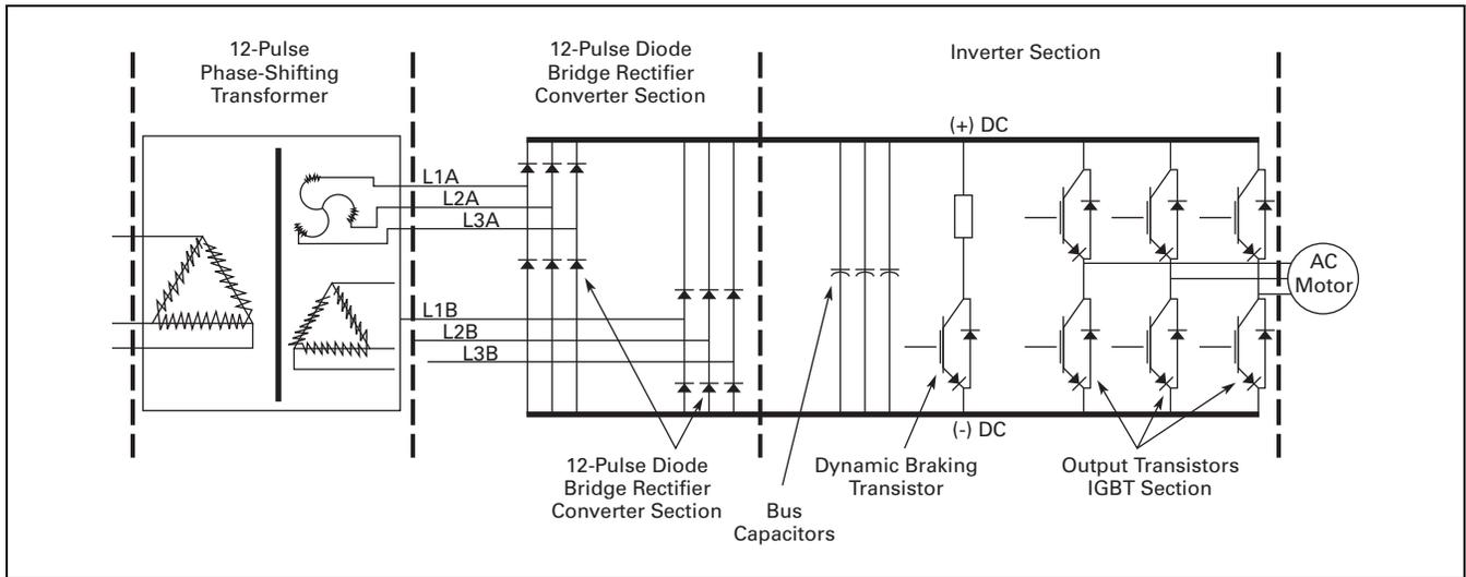
**Figure 31.0-14. Basic 12-Pulse Rectifier with “Phase-Shifting” Transformer**
