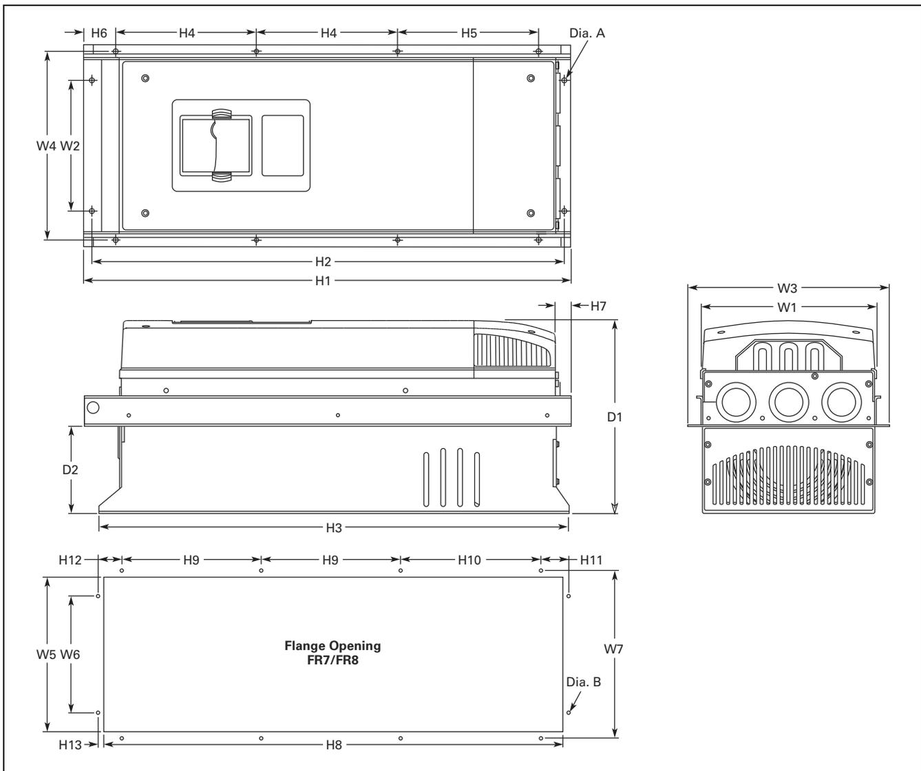
Figure 31.2-6. NEMA Type 1/IP21 and NEMA Type 12/IP54, with Flange Kit, FR7 and FR8
