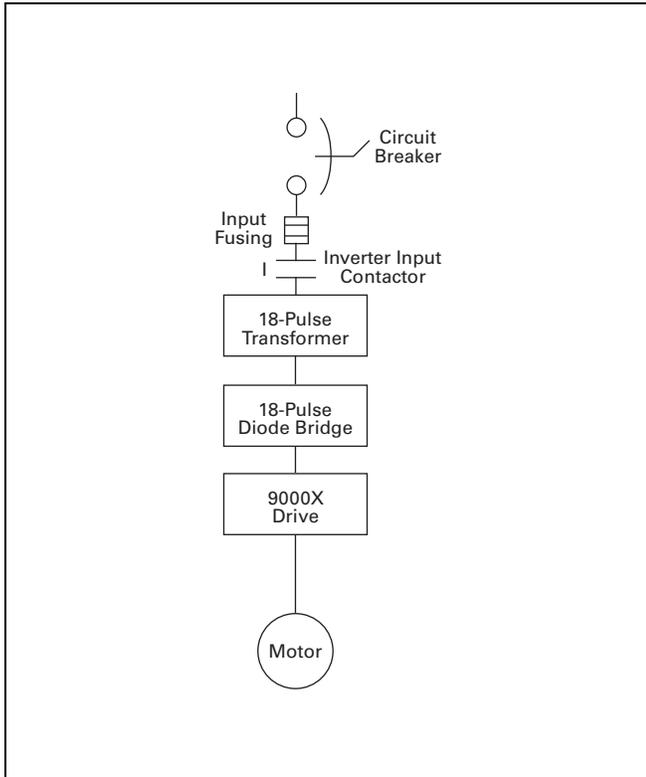
Figure 31.2-47. Power Diagram 25–250 hp  $I_L$  and 25–200 hp  $I_H$
