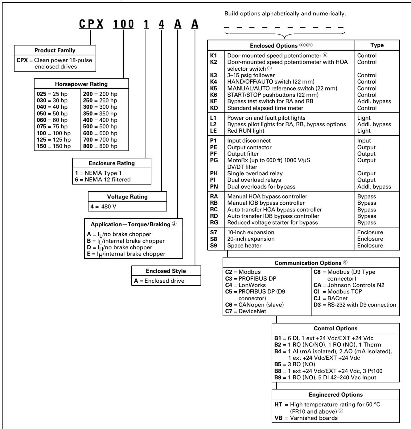
① Brake chopper is standard in drives up to 30 hp I<sub>H</sub> or 40 hp I<sub>L</sub>. It is optional in larger drives.
