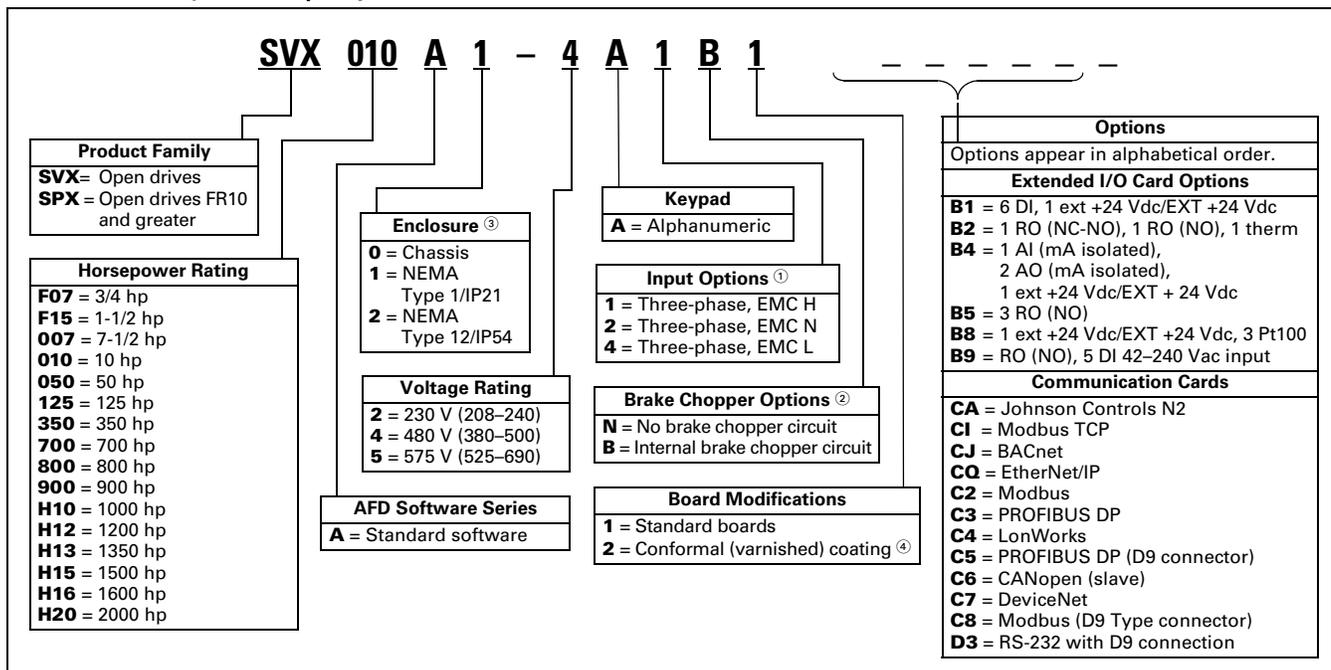
① All 230 V drives and 480 V drives up to 200 hp (IH) are only available with input option **1** (EMC Level H). 480 V drives 250 hp (IH) or larger are available with input option **2** (EMC Level N). 480 V drives are available with input option **4** (EMC Level L). 575 V drives 200 hp (IH) or larger are only available with input option **2**. 575 V drives up to 150 hp (IH) are only available with input option **4** (EMC Level L).
