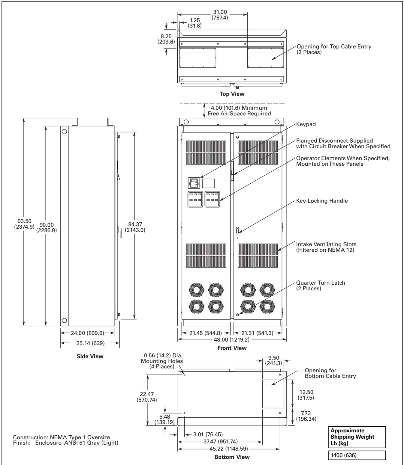
**Figure 31.2-41. Enclosure Size 8—Approximate Dimensions in Inches (mm)**
