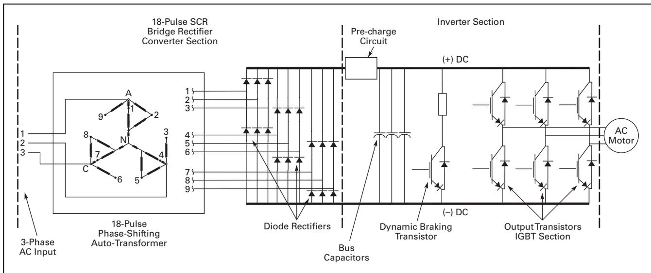
**Figure 31.0-16. Basic 18-Pulse Rectifier with Phase-Shifting Auto-Transformer**
