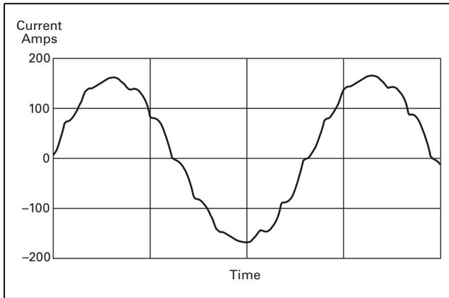
**Figure 31.0-13. 100 hp 480 V Drive with 12-Pulse Rectifier**
