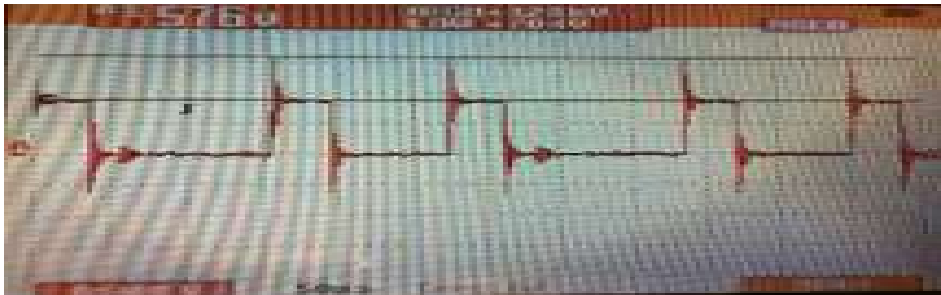
PWM at motor without dV/dT Filter
