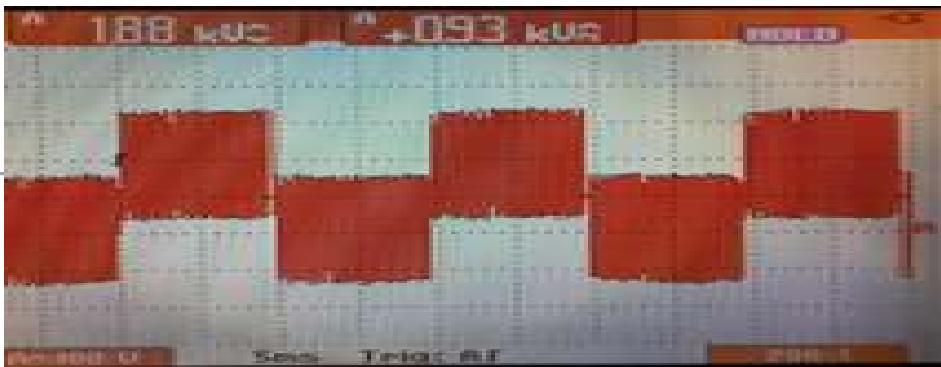
PWM at motor with dV/dT Filter
