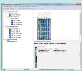
Offline functions, including the ability to configure and test systems, generate a bill of material, and create device specifications are just as helpful during commissioning and installation as online "signal state reading and setting" functions.
