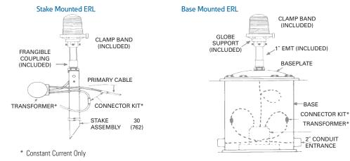
Note: All ERL 6.6A versions include a lead with L-823 plug. All ERL 120v versions have wire leads without connectors.
