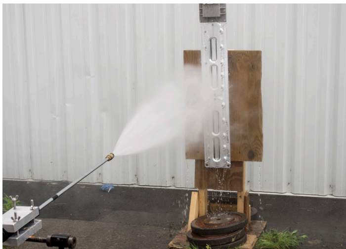
Pauluhn ZPLA tested to withstand 2,000 psi hose test at 5 ft. distance
