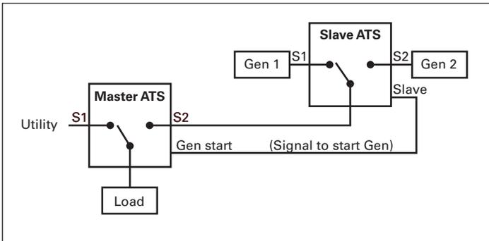
Figure 9. Three-source transfer switch arrangement
