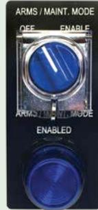
Prior to performing maintenance, service personnel can enable ARMS via a lockable selector switch (blue) that can be incorporated into a lockout/tagout (LOTO) procedure. A corresponding blue light provides visual indication that the ARMS maintenance mode is enabled.
