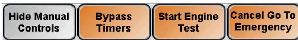
The “Show Manual Controls” button expands a small area with 3 control buttons: Go to Emergency, Bypass Timers, and Start Engine Test. All control is password protected except Bypass Timers. To hide the manual controls, press the “Hide Manual Controls” button.
