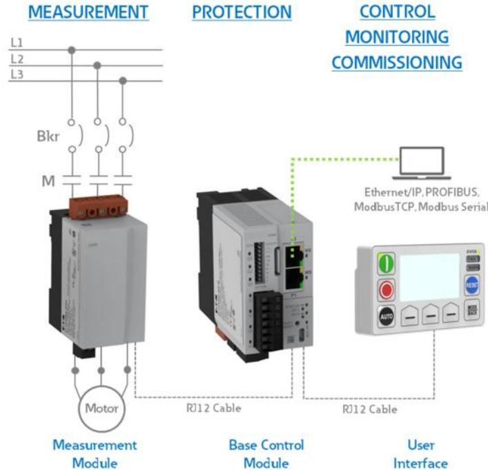
Fig. 1 Typical microprocessor based motor management relay
