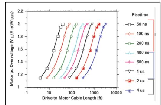
**Figure 1. Cable Length Versus Overvoltage [2]**
