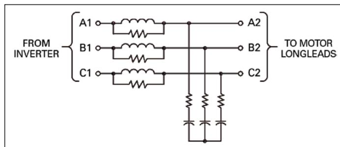
Figure 2. dV/dT Filter Schematic [3]
