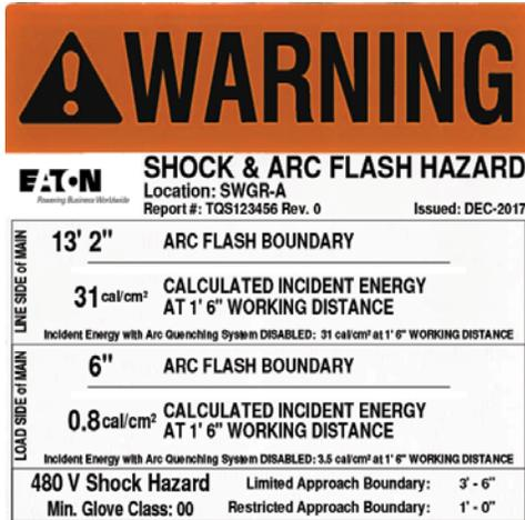
Figure 3. Sample arc flash label for AQD on load-side of LV main breaker
