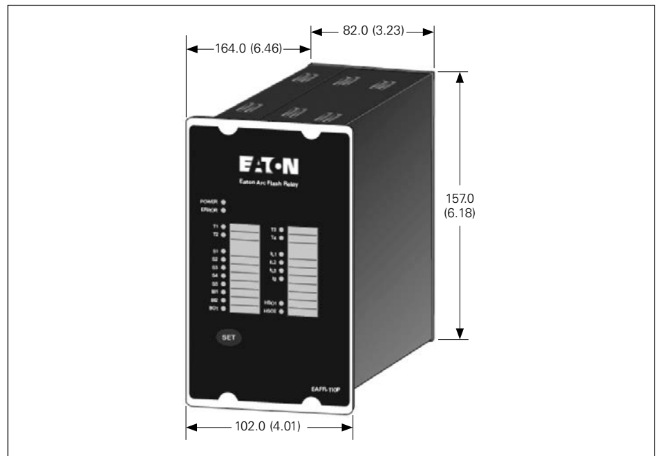
Figure 20.5-5. EAFR-110PLV Dimensions in Millimeters (Inches)
