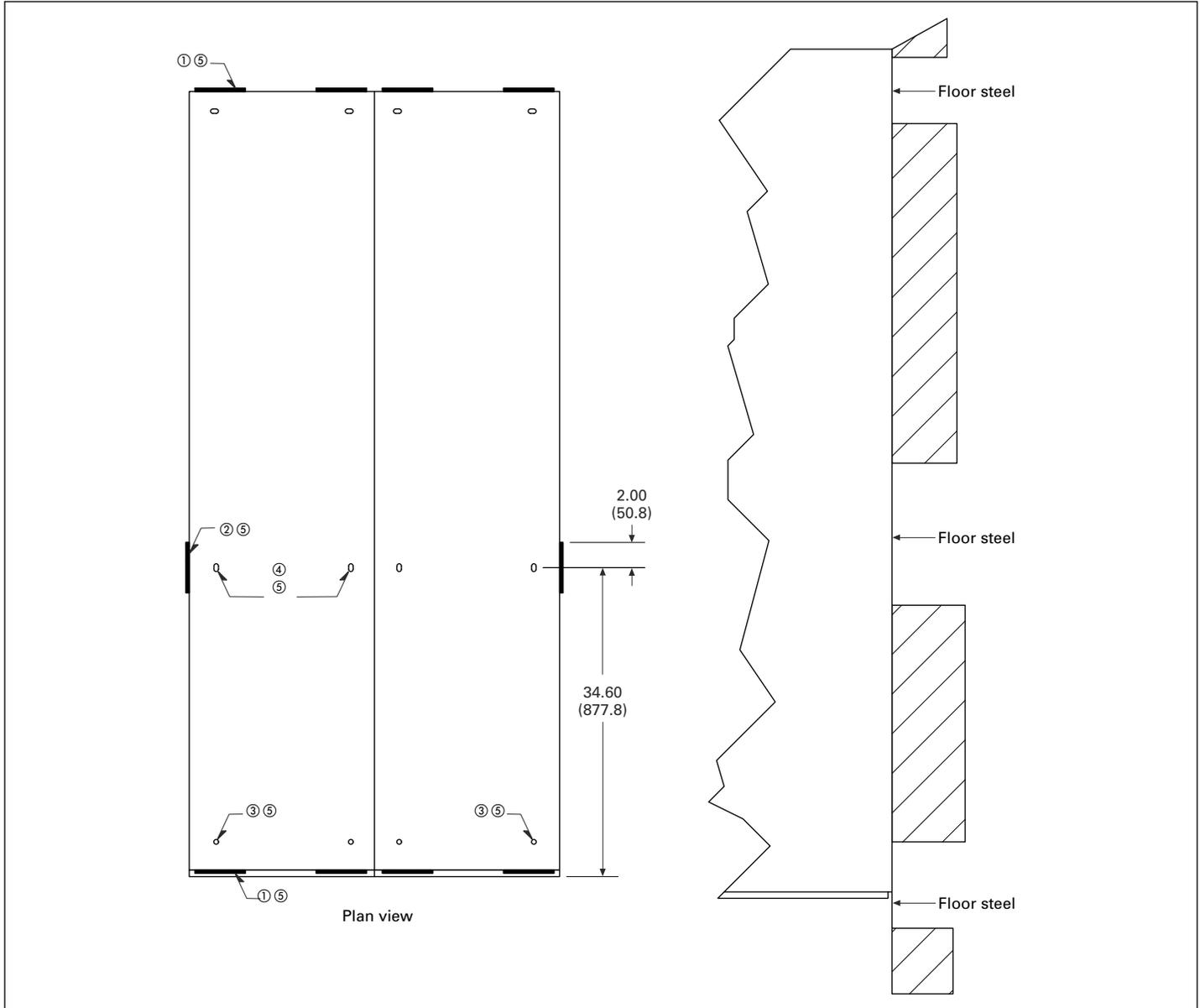
**Figure 1. Welding of indoor structures to imbedded floor steel—rear-access MDS, MDN, MSB, and Series NRX®**
