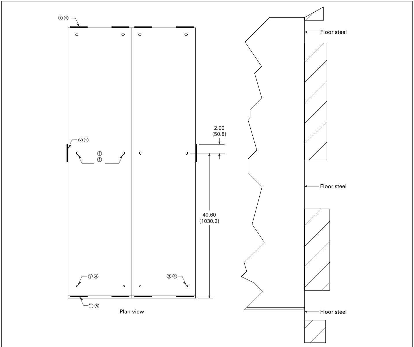
**Figure 2. Welding of indoor structures to imbedded floor steel—rear-access MDSL**
