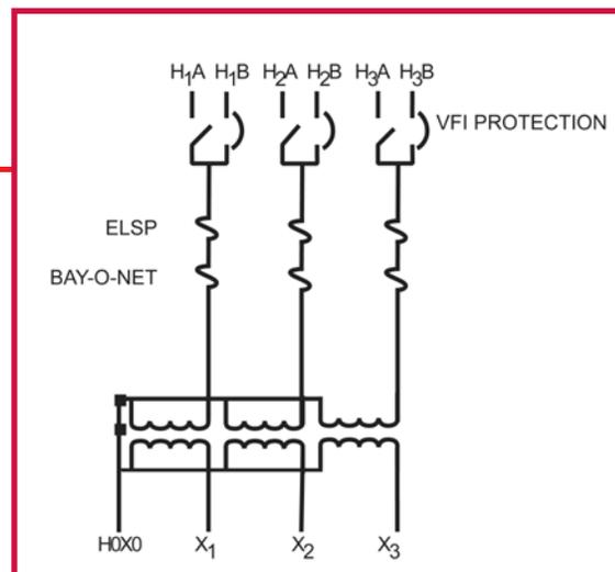
How To Specify “Transformer shall be an Eaton liquid-filled transformer designed in accordance with the requirements of IEEE Std C57.12.00™ standard. The overcurrent protection shall be provided with a Cooper Power series Vacuum Fault Interrupter (VFI) integral to the transformer tank. The VFI electronic breaker shall have a maximum interrupting rating of 12,500 A RMS symmetrical with resettable fault protection up through 35 kV.”
