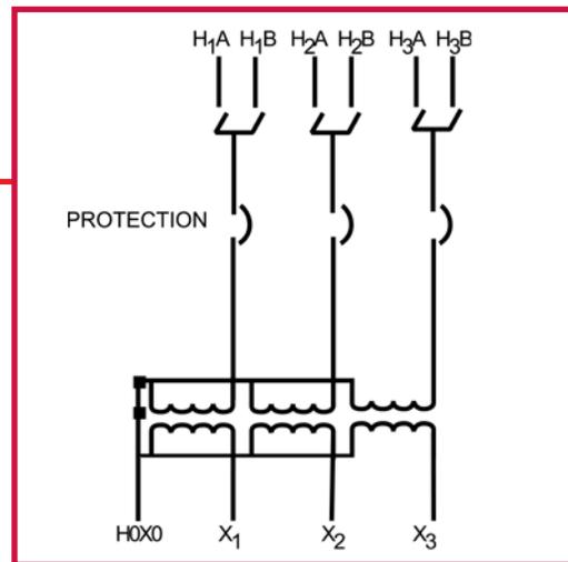
Schematic B: Three-phase VFI transformer with loop protection
