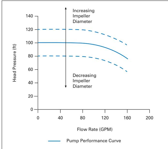
**Figure 1. Impeller Diameter Impact on Pump Performance Curve**
