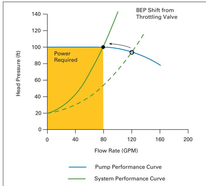
**Figure 3. Throttling Valve Impact on Pump System BEP**
