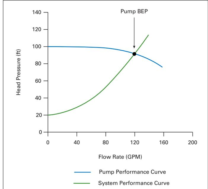
**Figure 2. Pump System Best Efficiency Point (BEP)**
