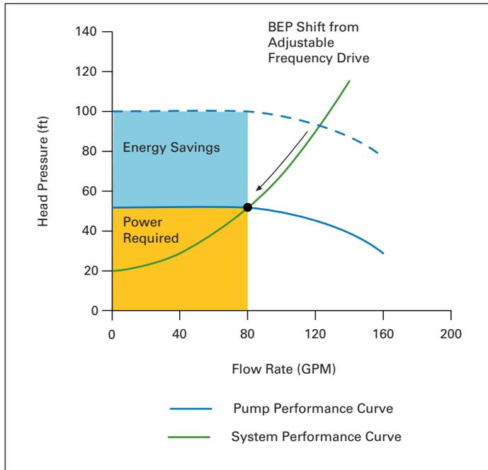
**Figure 4. Variable Frequency Drive Impact on BEP**
