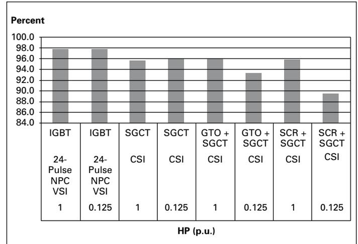
Figure 10. Drive Efficiency
