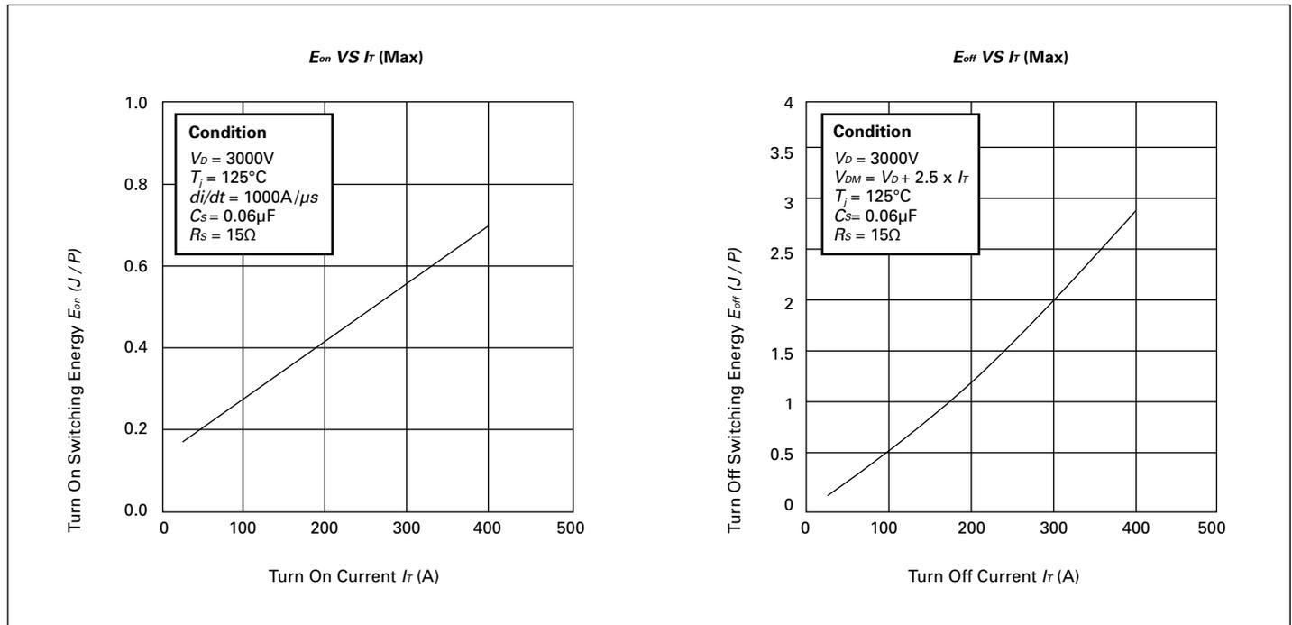
Figure 8. SGCT Switching Losses ③
