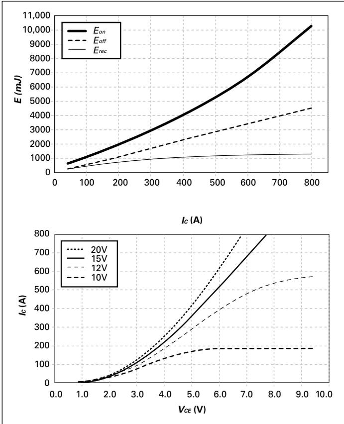
Figure 9. IGBT Switching and Conduction Losses ⑥
